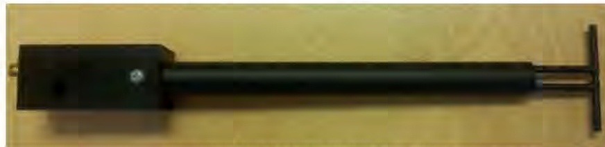
Figure 1 – MVG COMOSAR Validation Dipole
