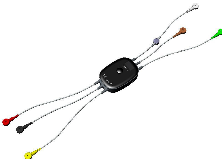
Figure 3-9 Wireless FECG Fetal&Maternal Module and ECG Leads
