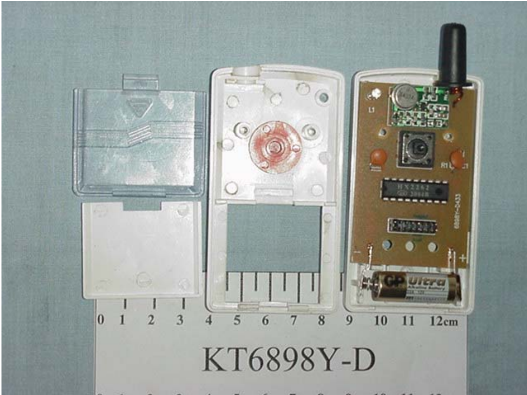
FIGURE 1 WIRELESS DOOR CHIME (M/N: KT6898Y-D) COVER REMOVED
