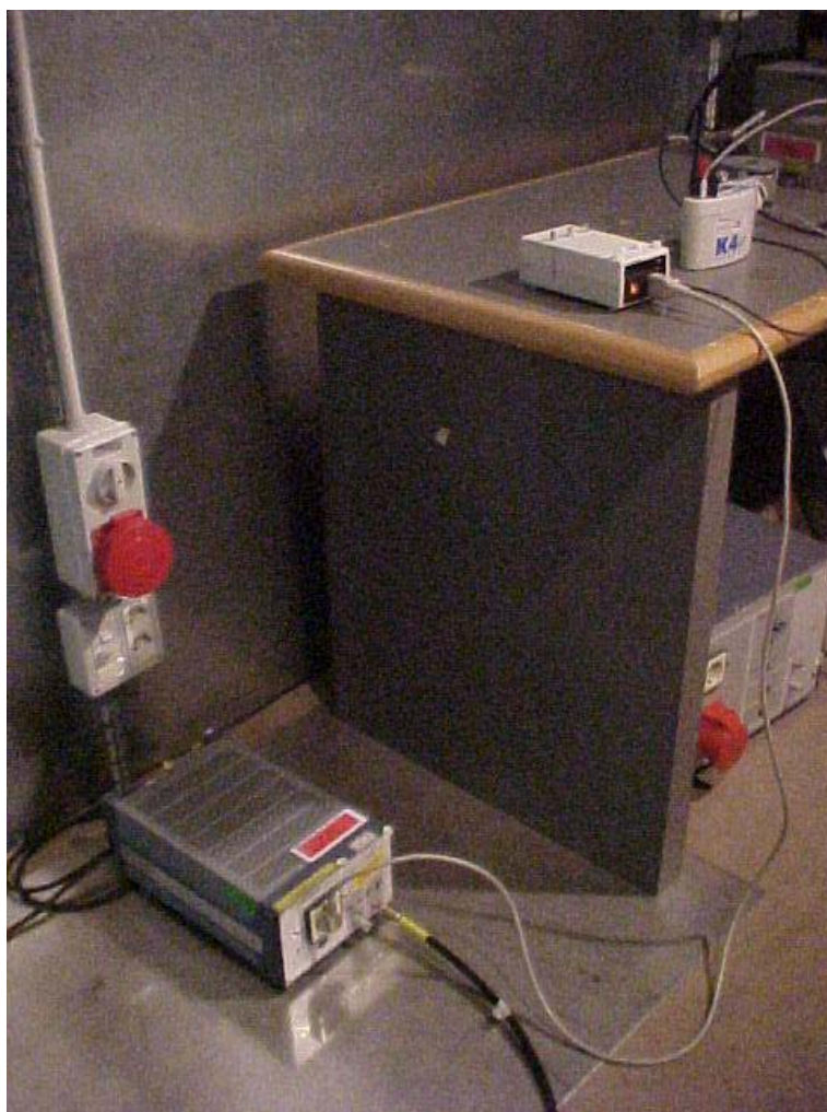
PHOTO N° 5 – SET-UP FOR EMISSION CONDUCTED TEST
