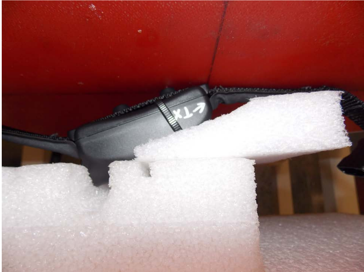
Test Position Main Antenna 0 mm Gap
