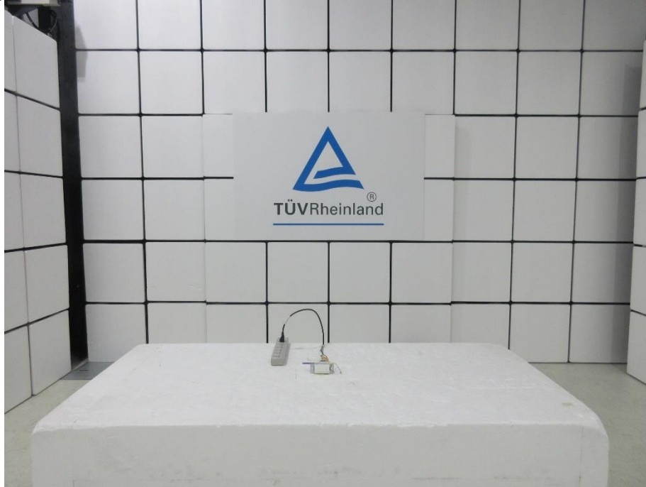
Photograph 1: Test Setup for Spurious Emissions (Front View 1)
