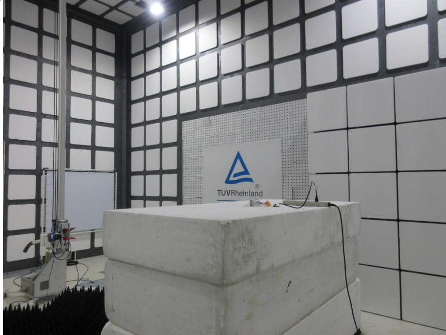
Photograph 5: Test Setup for Spurious Emissions (Back View 3)
