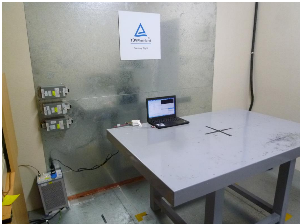
Photograph 7: Set-up for for Mains Conducted testing Front
