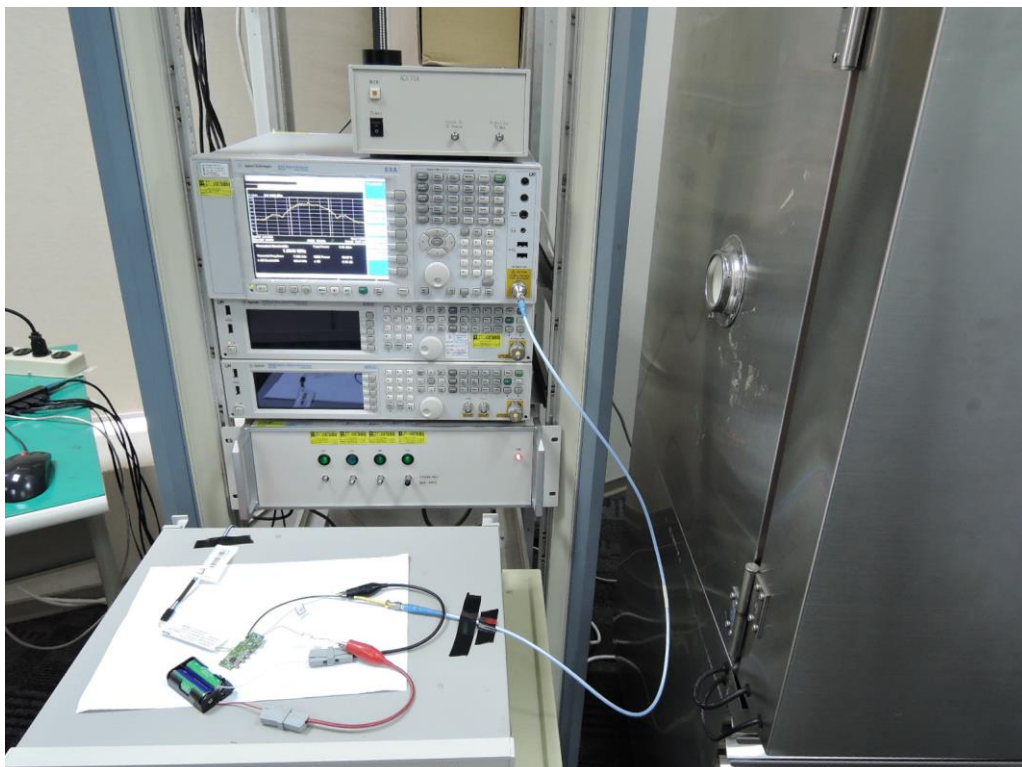
Photograph 5: Set-up for Conducted testing
