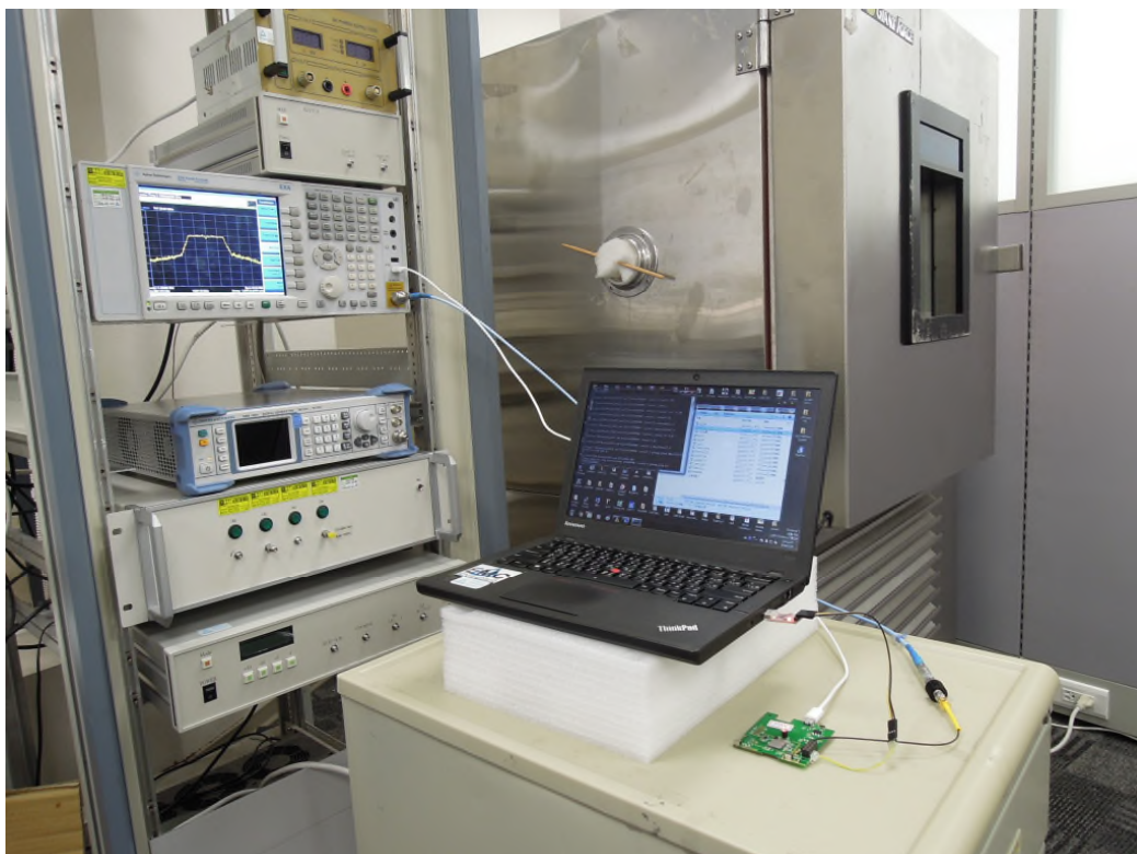
Photograph 4: Set-up for Conducted testing
