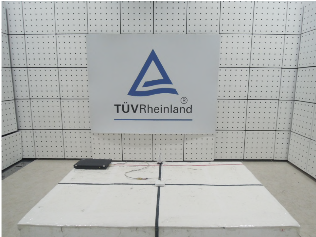
Photograph 2: Set-up for Spurious Emissions (Back View 1)
