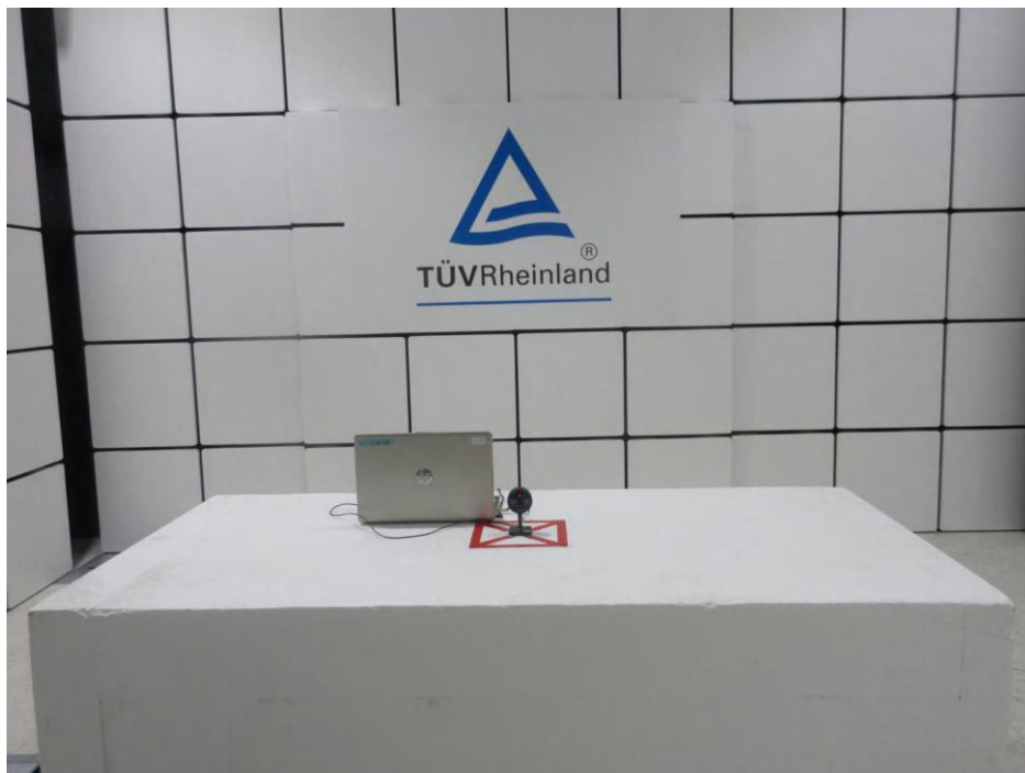
Photograph 2: Set-up for Spurious Emissions (Front View 2)
