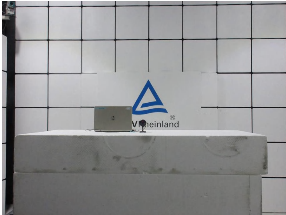
Photograph 1: Set-up for Spurious Emissions (Front View 1)
