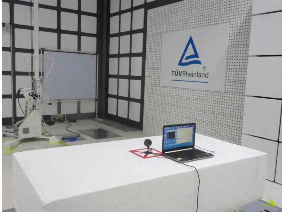
Photograph 5: Set-up for Spurious Emissions (Back View 3)
