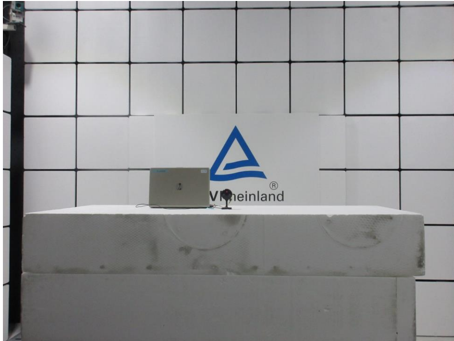
Photograph 1: Set-up for Spurious Emissions (Front View 1)
