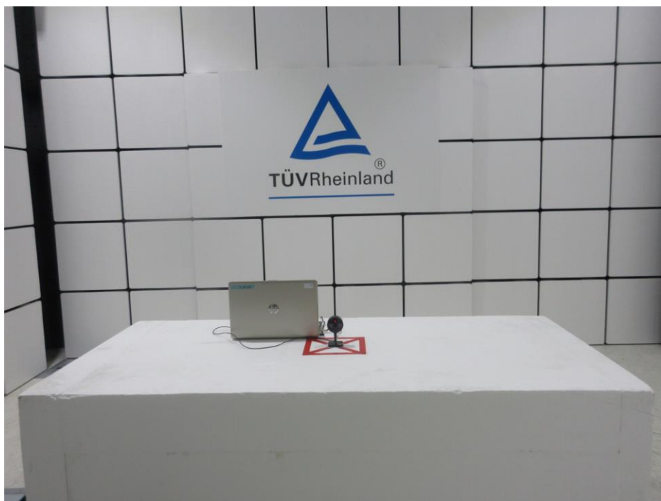
Photograph 2: Set-up for Spurious Emissions (Front View 2)
