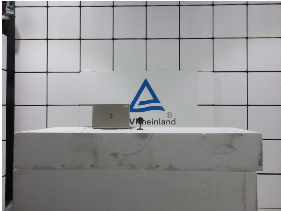
Photograph 1: Set-up for Spurious Emissions (Front View 1)
