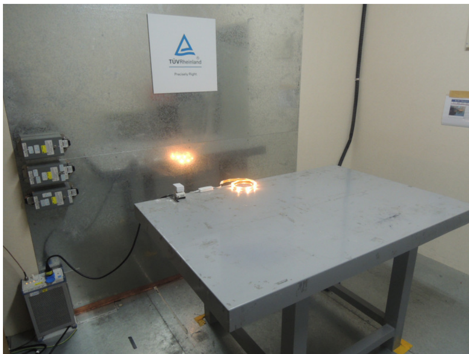
Photograph 8: Set-up for Mains Conducted testing (Front View)
