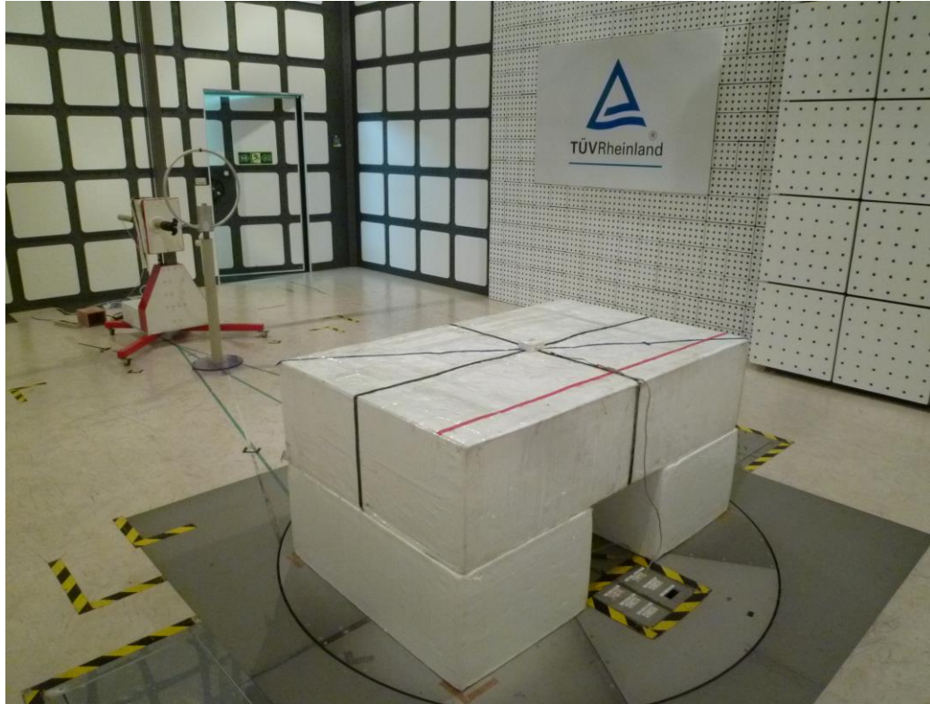
Photograph 5: Set-up for Conducted testing
