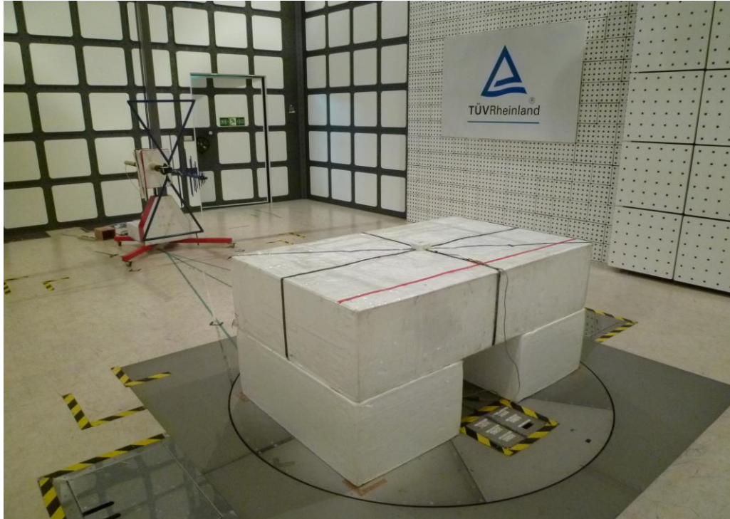
Photograph 2: Set-up for Spurious Emissions (Back View 1)
