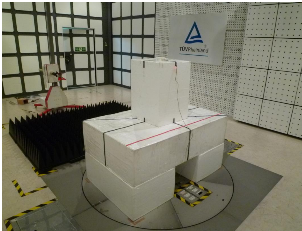
Photograph 3: Set-up for Spurious Emissions (Back View 2)
