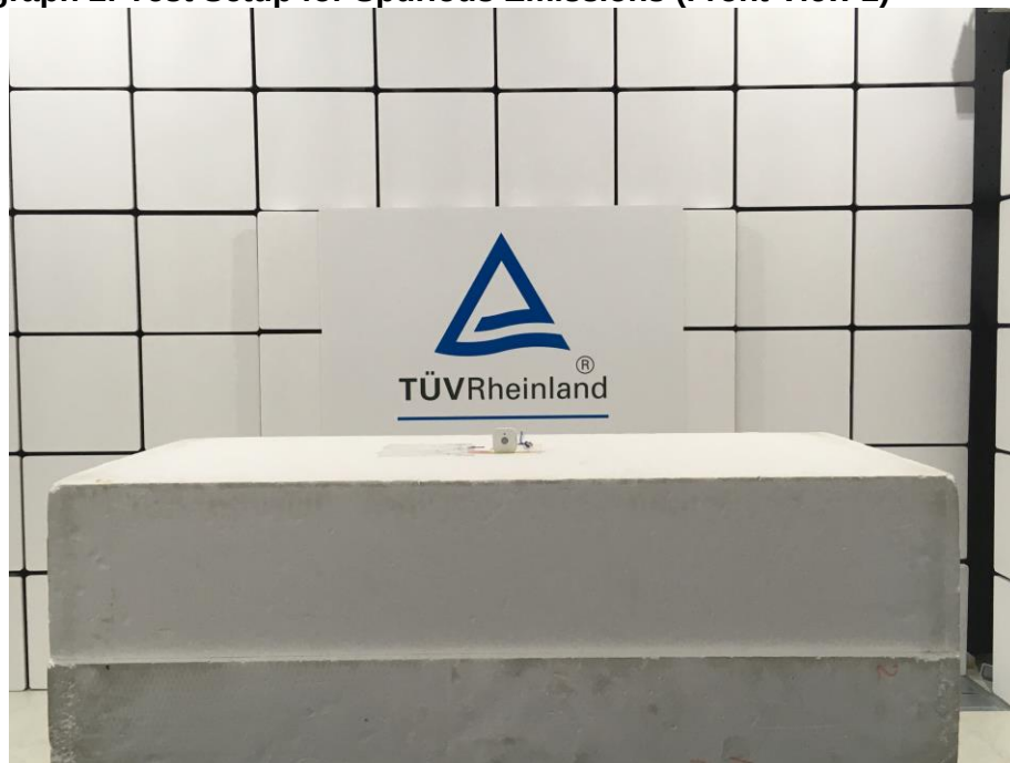
Photograph 2: Test Setup for Spurious Emissions (Front View 2)
