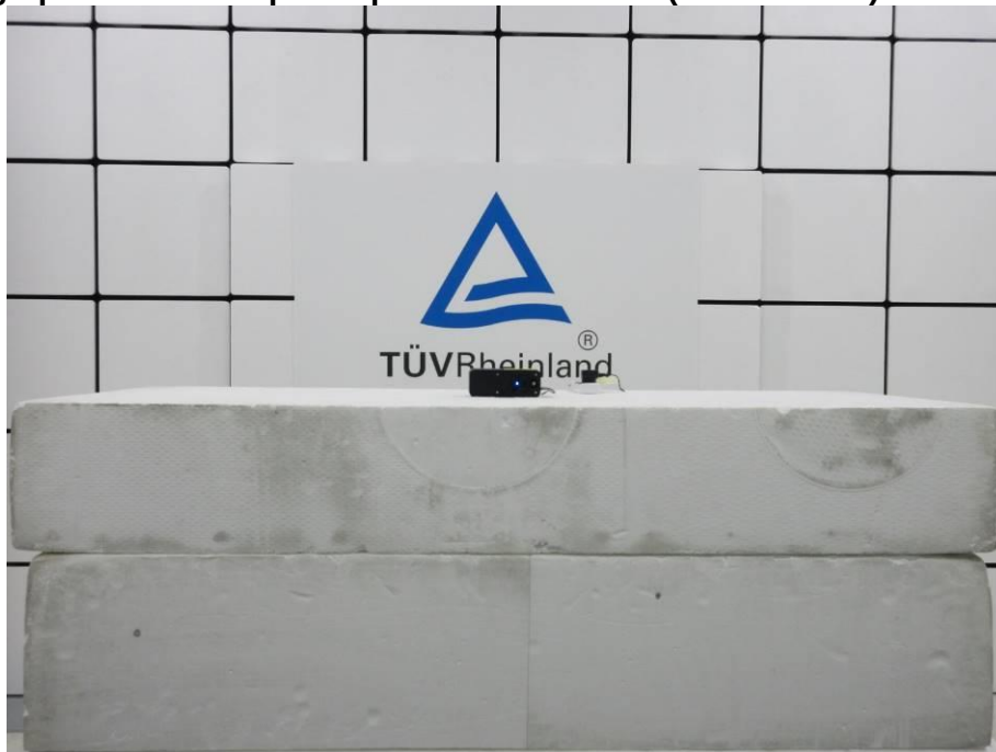
Photograph 2: Test Setup for Spurious Emissions (Front View 2)
