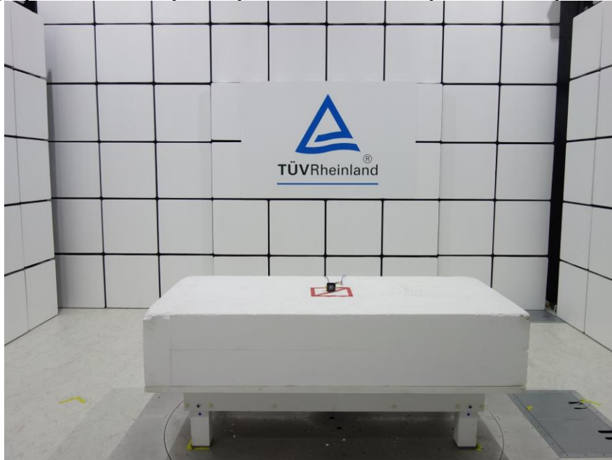
Photograph 1: Test Setup for Spurious Emissions (Front View 1)
