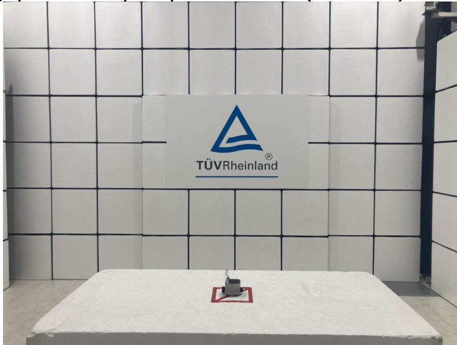
Photograph 1: Test Setup for Spurious Emissions (Front View 1)
