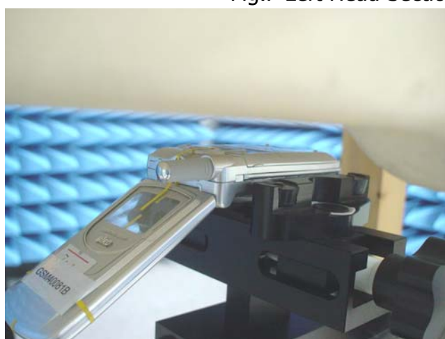
Fig.7 Left Head Section / Ear-Tilt Position(15°)
