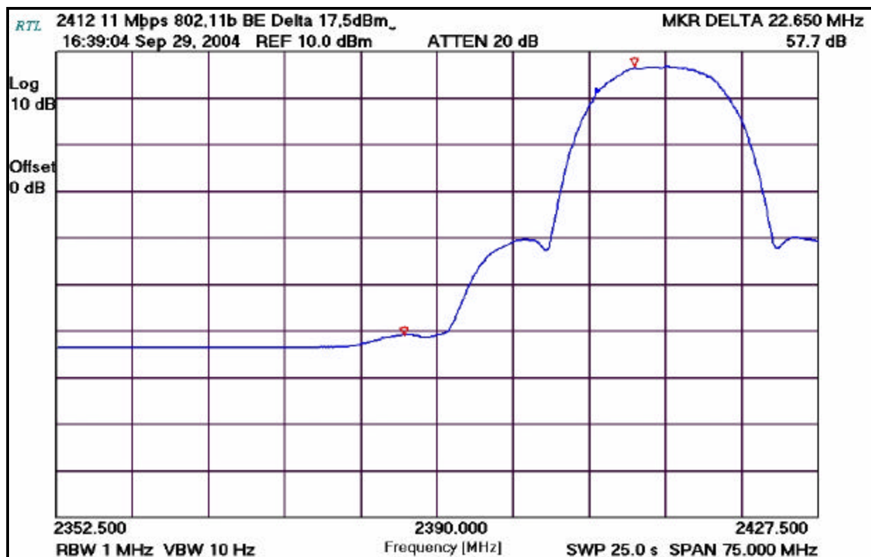
PLOT 4-15: LOWER BAND EDGE: AVERAGE MEASUREMENT CHANNEL 1 (TX FREQUENCY: 2412 MHZ – 11 MB/S)
