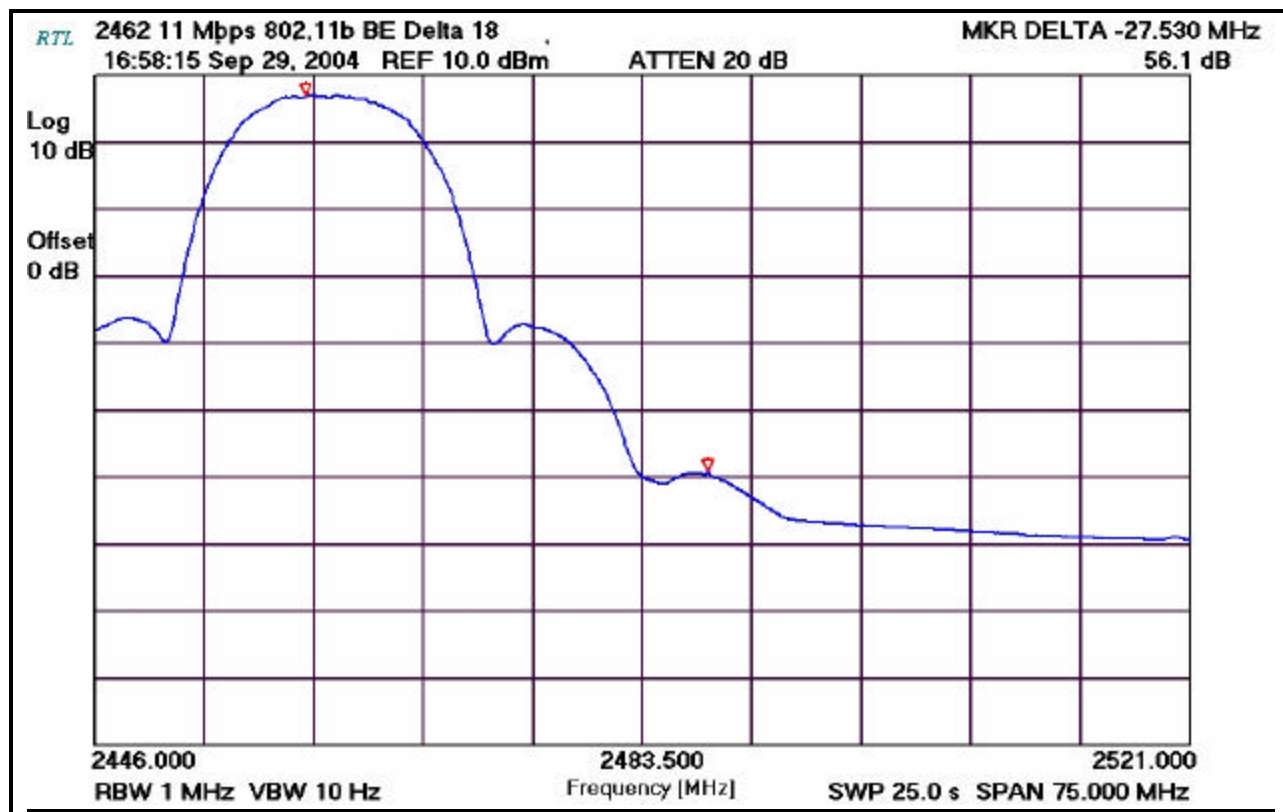
PLOT 4-16: UPPER BAND EDGE: AVERAGE MEASUREMENT CHANNEL 11 (TX FREQUENCY: 2462 MHZ – 11 MB/S)
