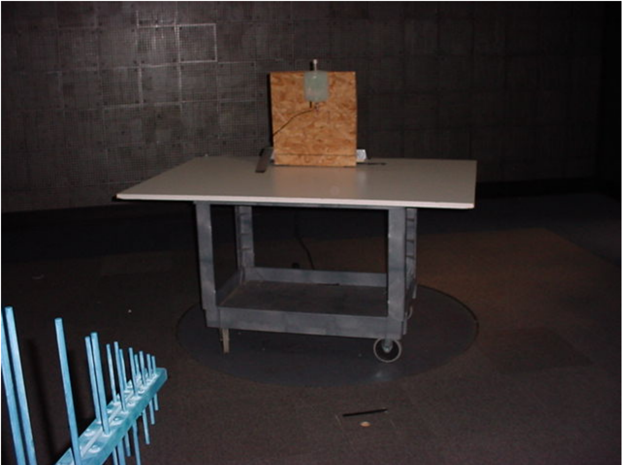
Figure 1: Unintentional Radiated Emissions –Front View
