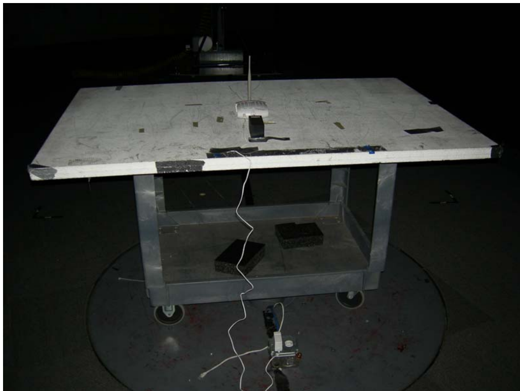
Figure 5: Test Setup – Unintentional Radiated Emissions
