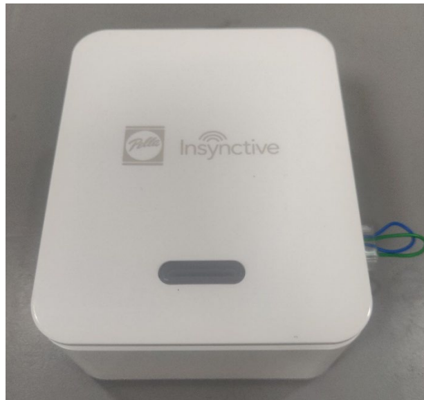
Figure 1: Photograph of Pella Insynctive Bridge- Full View
