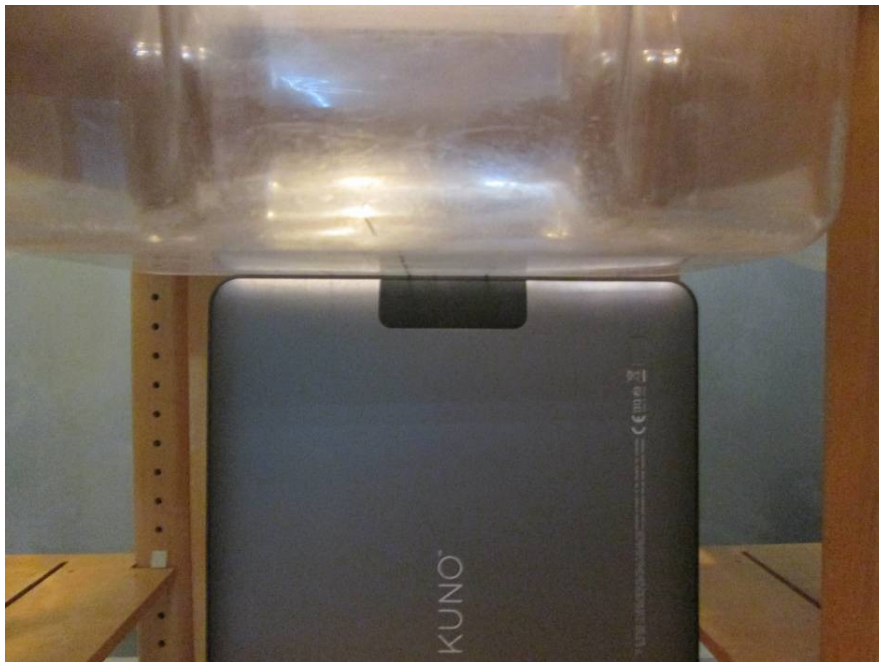
Body-Left Setup Photo (0.0mm)
