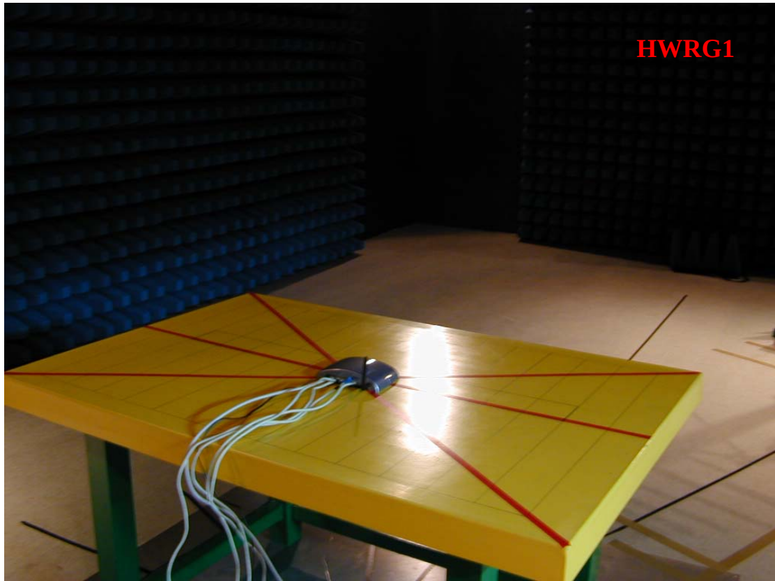
Photo 2: Radiated Emission Test Set-up
