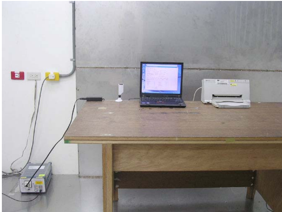
Photo 2: Conducted Emission Test Set-up
