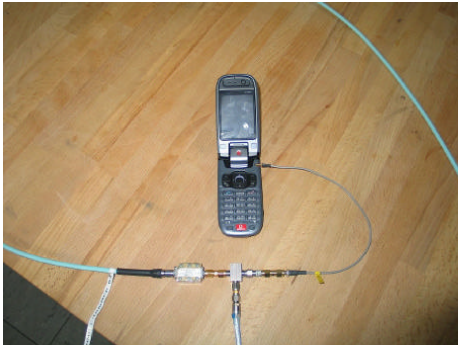
Picture 2 : Setup for conducted tests
