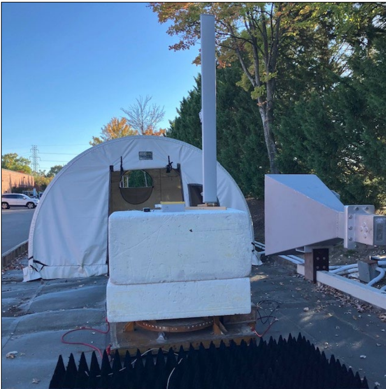
Photograph 11: Radiated Emissions – Front View – Sector Antenna Greater Than 1 GHz – FMN
