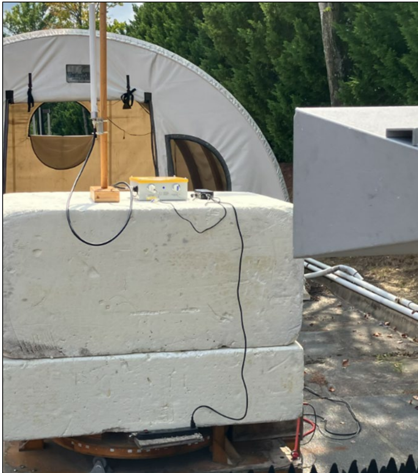
Photograph 6: Radiated Emissions – Rear View – Omni Antenna Greater Than 1 GHz
