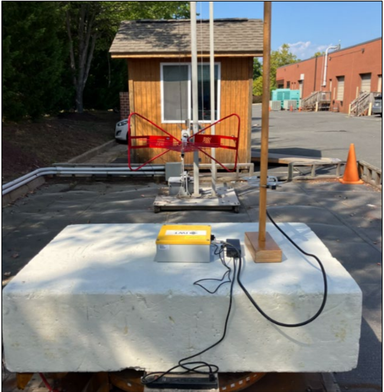
Photograph 4: Radiated Emissions – Rear View – Yagi Antenna Less Than 1 GHz
