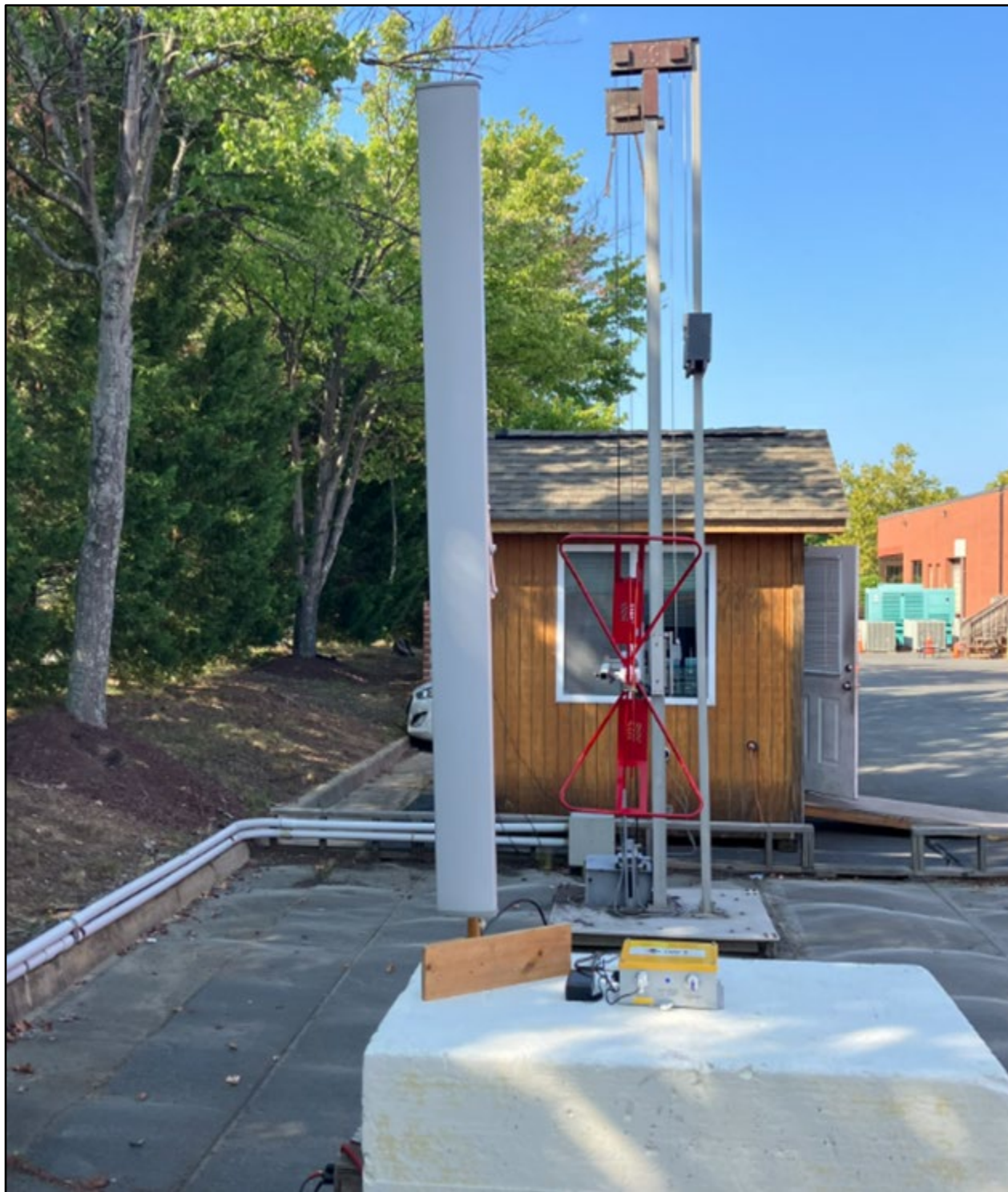
Photograph 13: Radiated Emissions – Front View – Sector Antenna Less Than 1 GHz – GWN
