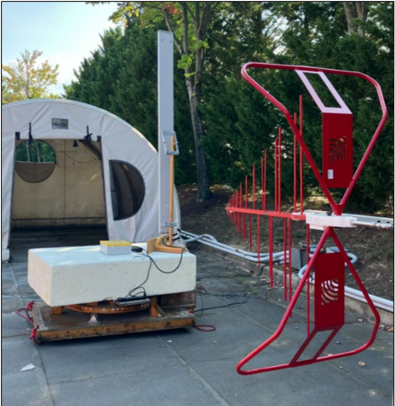
Photograph 2: Collocated Radiated Emissions – Rear View – Sector Antenna
