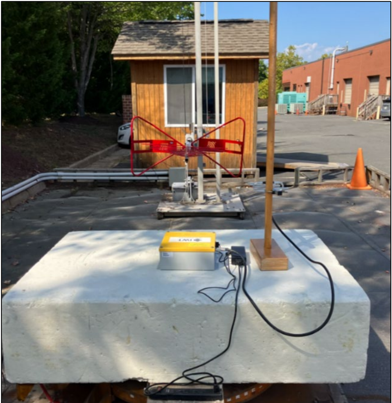
Photograph 4: Collocated Radiated Emissions – Rear View – Yagi Antenna
