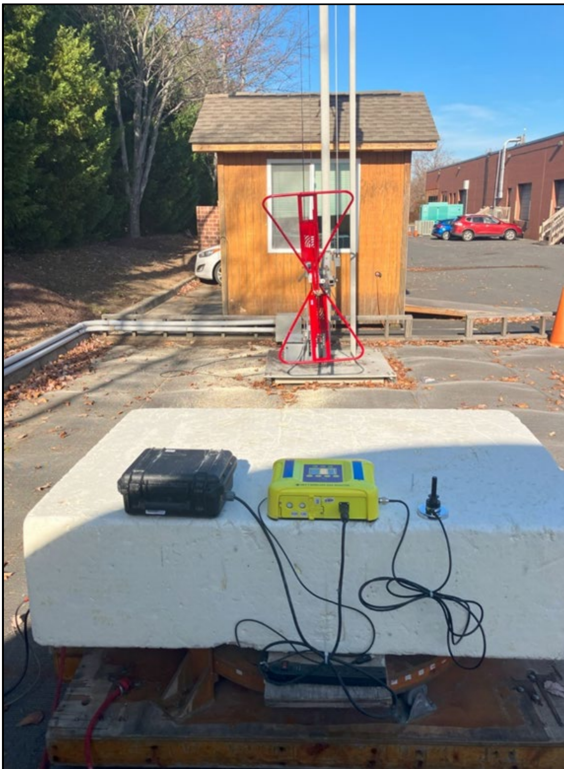
Photograph 6: Unintentional Radiated Testing – Back (Below 1 GHz) Omni Antenna
