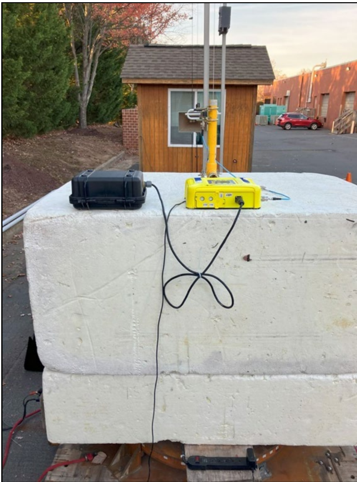
Photograph 4: Radiated Testing – Back (Above 1 GHz) Yagi Antenna
