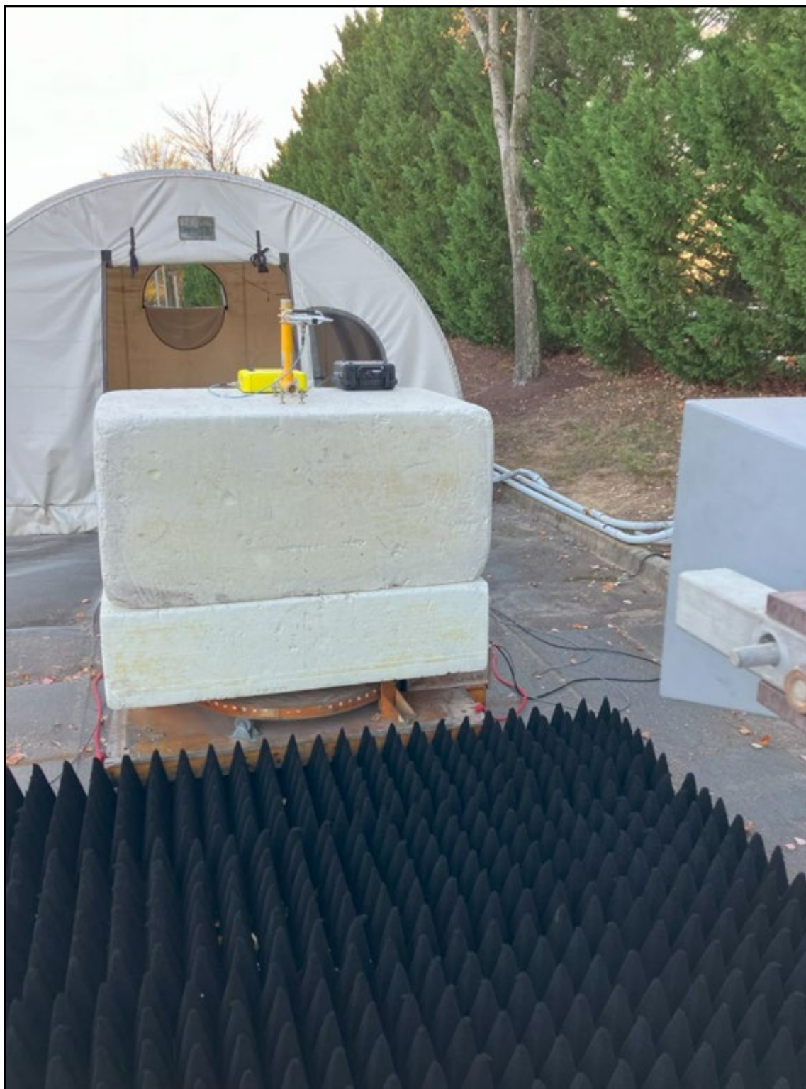
Photograph 3: Radiated Testing – Front (Above 1 GHz) Yagi Antenna
