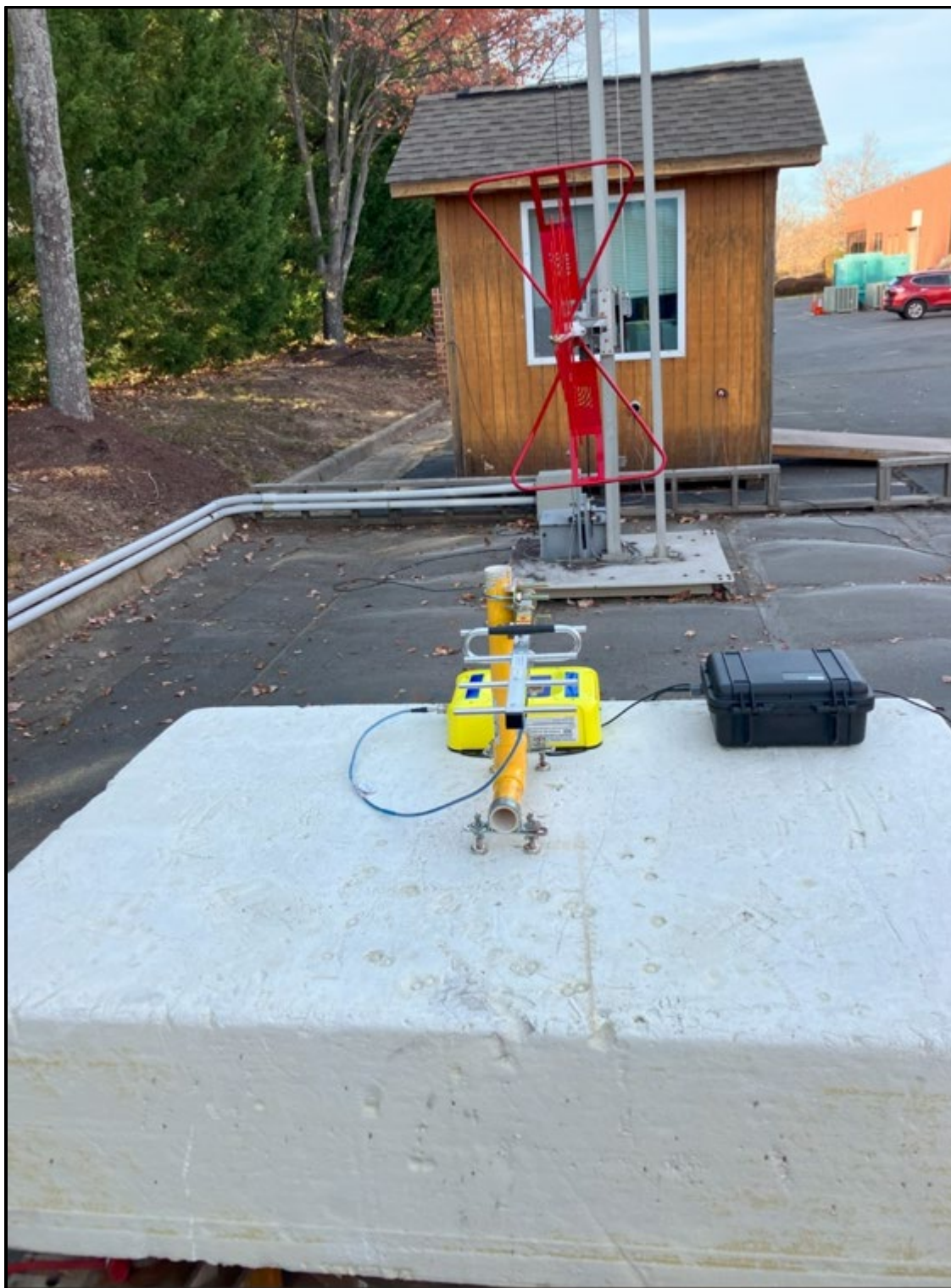
Photograph 2: Radiated Testing – Back (Below 1 GHz) Yagi Antenna
