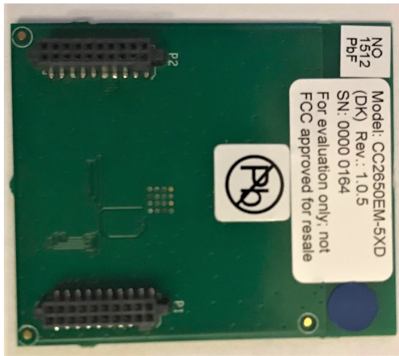
TEXAS INSTRUMENTS CC2650EM-5XD BOTTOM VIEW
