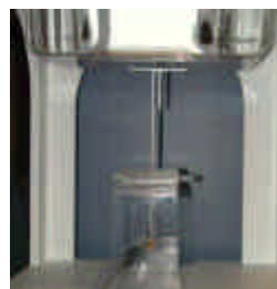
Figure A.0 Dipole Validation Test Setup
