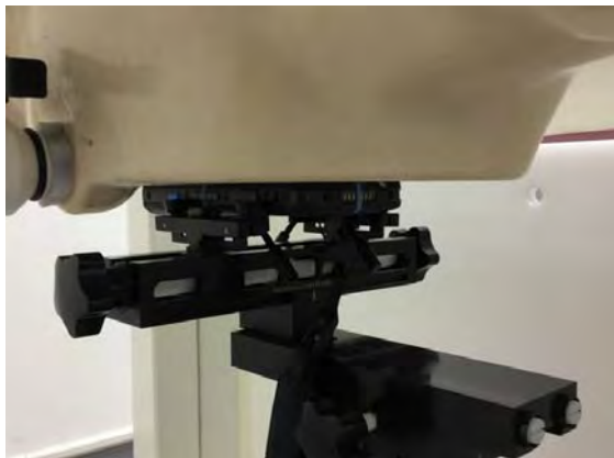
Fig.9 EUT Front side to flat phantom
