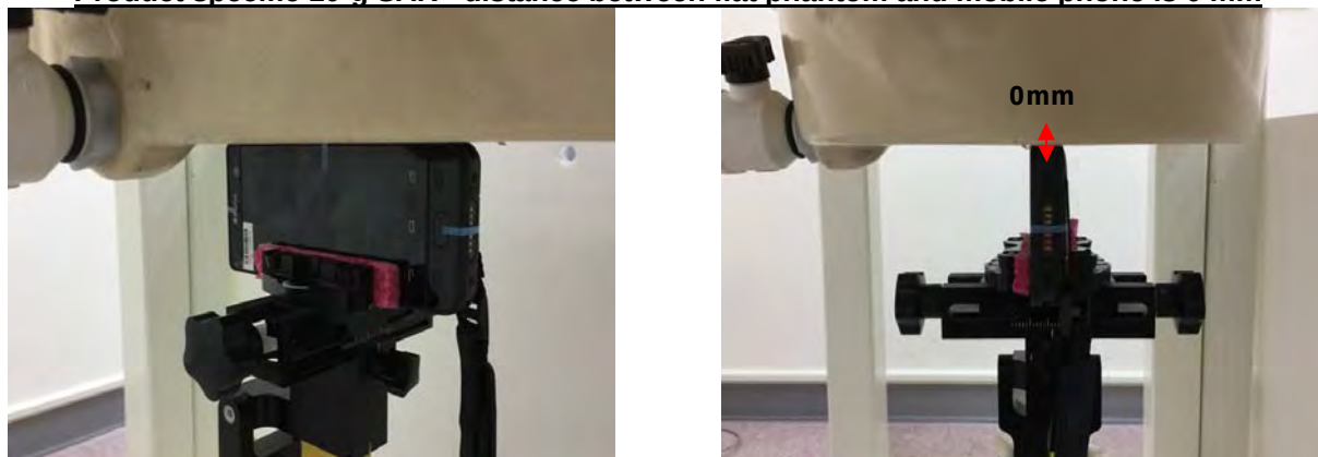
Fig.12 EUT Right side to flat phantom
