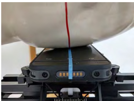
Fig.5 Left Head Section / Cheek-Touch Position
