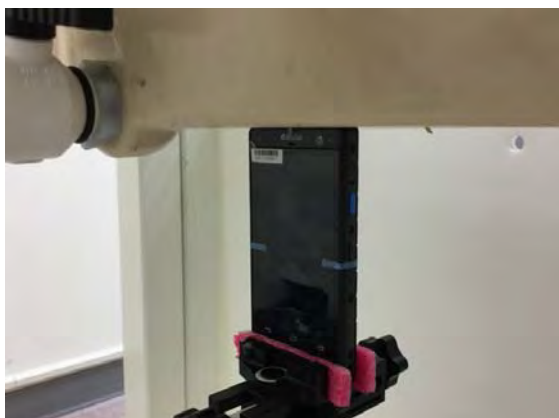
Fig.11 EUT Top side to flat phantom
