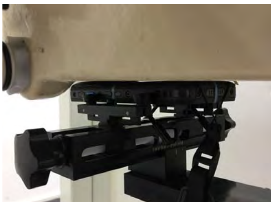
Fig.10 EUT Back side to flat phantom
