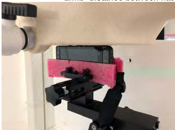
Fig.18 EUT Right side to flat phantom
