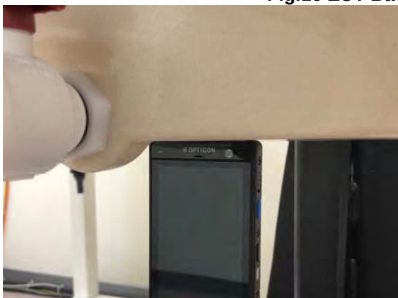
Fig.17 EUT Top side to flat phantom
