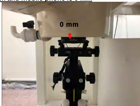
Fig.15 EUT Front side to flat phantom
