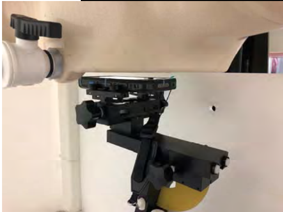
Fig.7 EUT Front side to flat phantom
