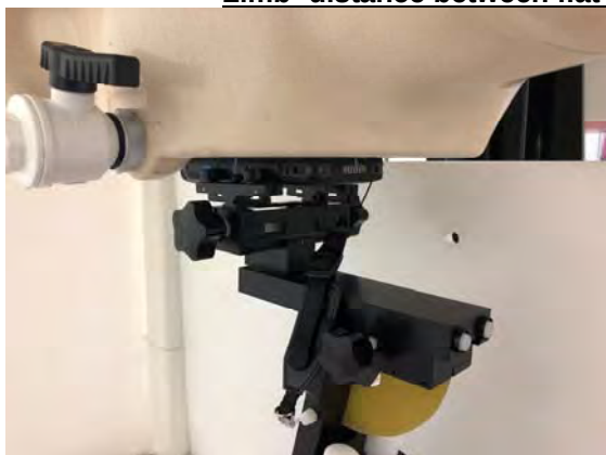
Fig.15 EUT Front side to flat phantom
