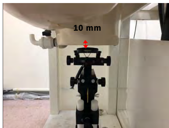
Fig.10 EUT Back side to flat phantom
