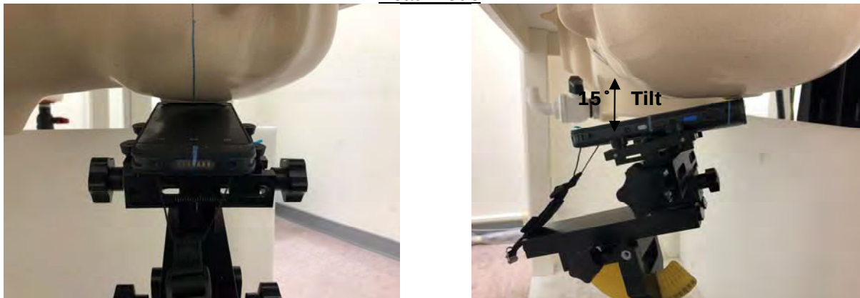
Fig.6 Left Head Section / Ear-Tilt Position(15°)
