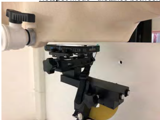
Fig.9 EUT Front side to flat phantom
