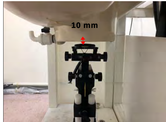
Fig.8 EUT Back side to flat phantom
