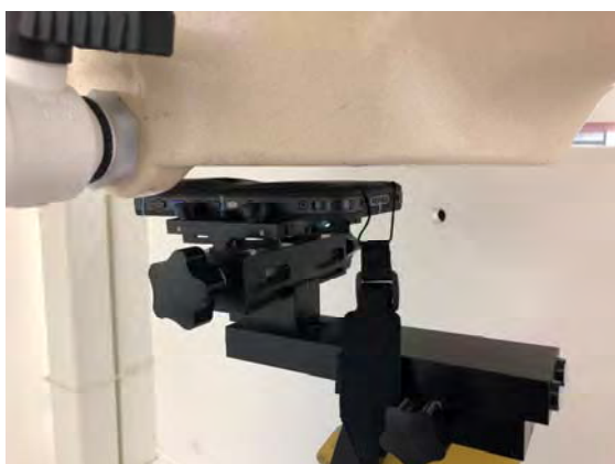
Fig.10 EUT Back side to flat phantom
