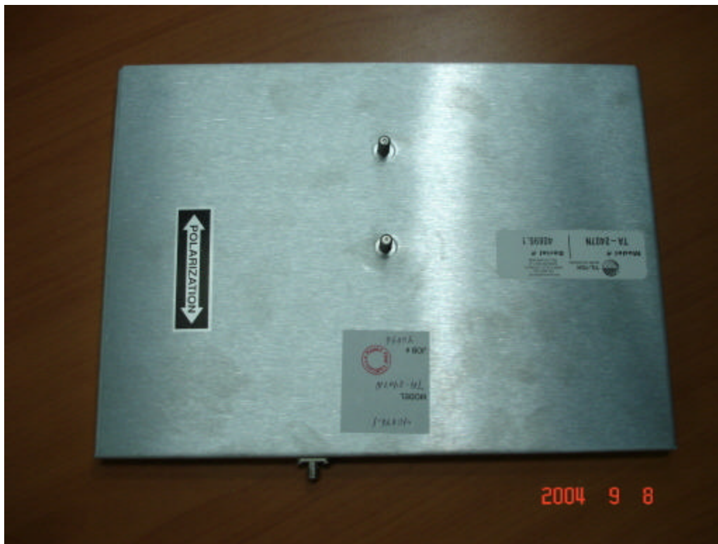
Flat panel antenna (NTA 2407)
