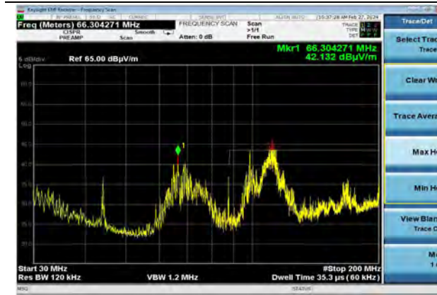
802.11a | Channel 36 | 6 Mbps | Y Plane 30-200 MHz | Vertical
