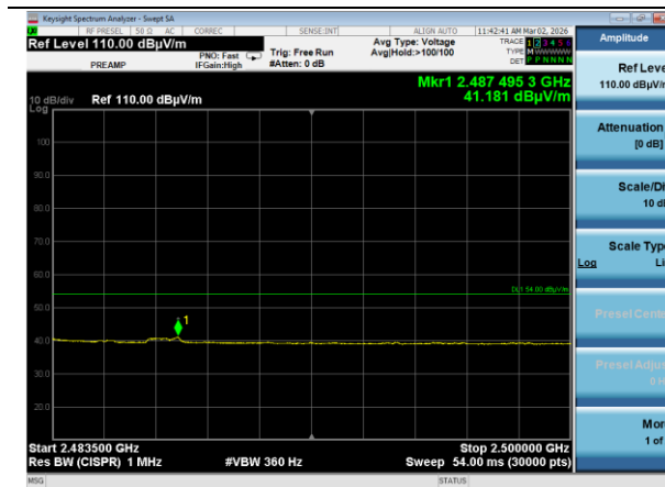
2483.5-2500 MHz Horizontal Average BTC 2DH5 Ch 78 Orientation 1
