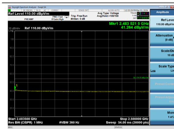
2483.5-2500 MHz Horizontal Average BTC 3DH5 Ch 78 Orientation 1
