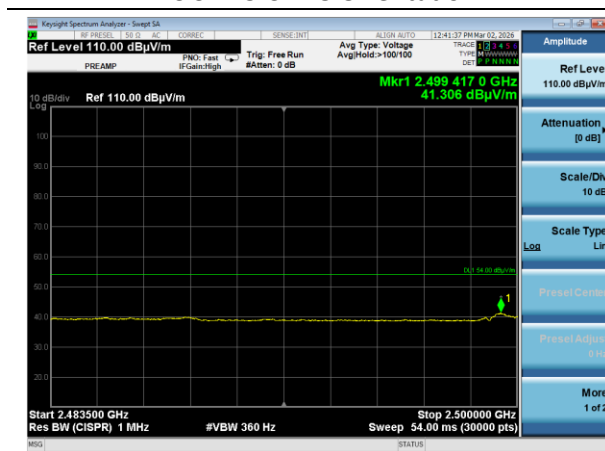
2483.5-2500 MHz Horizontal Average BTC DH5 Hopping Orientation 1
