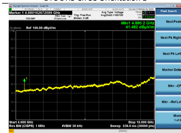
4000-18000 MHz Horizontal BTC DH5 Ch 38 Orientation 1
