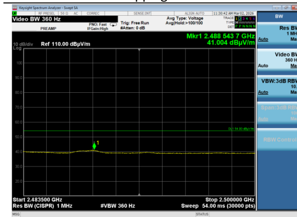
2483.5-2500 MHz Horizontal Average BTC DH5 Ch 78 Orientation 1
