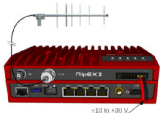
Fig. 4.8: 10–30 VDC Supplying
