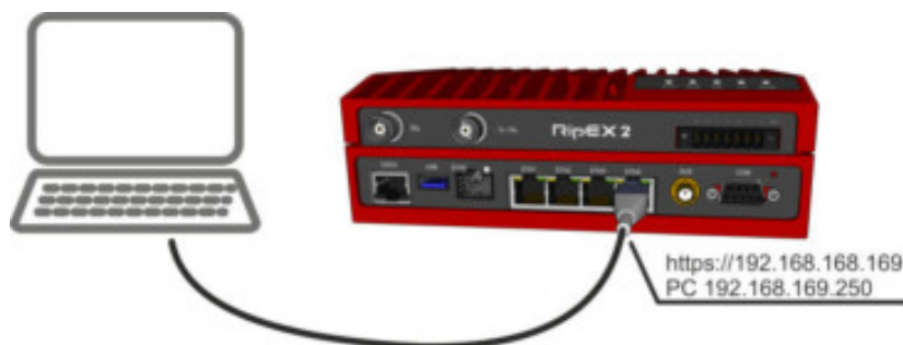
Fig. 3.6: Connecting to a PC over ETH
