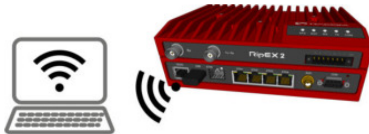
Fig. 3.4: Connecting to a PC over WiFi
