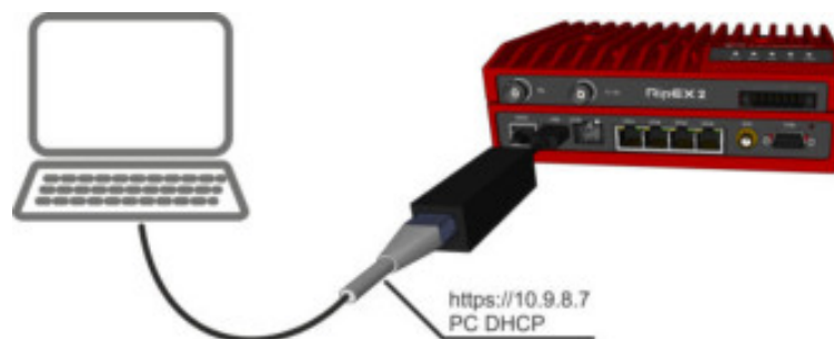
Fig. 3.5: Connecting to a PC over ETH/USB adapter
