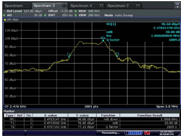
Figure 8.1-3: 20 dB Bandwidth, High CH
