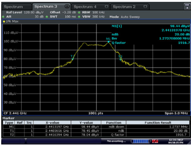
Figure 8.1-2: 20 dB Bandwidth, Mid CH
