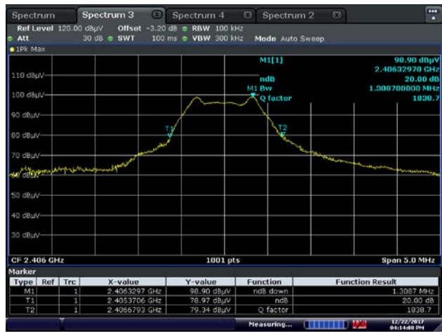
Figure 8.1-1: 20 dB Bandwidth, Low CH
