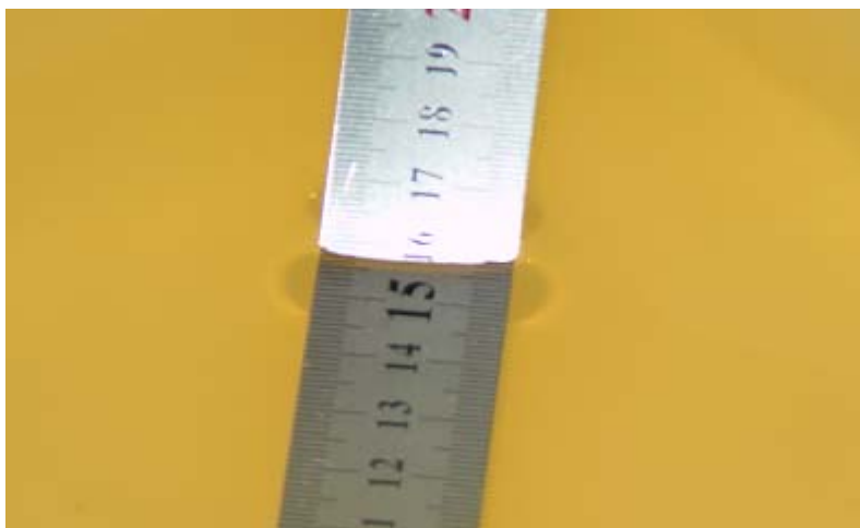
Liquid depth for SAR Measurement
