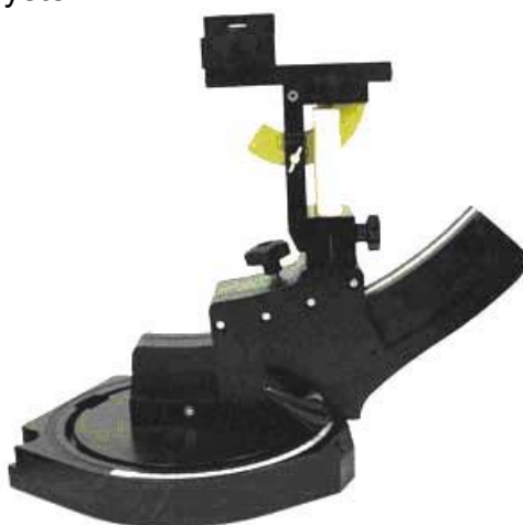
Device holder supplied by SPEAG
