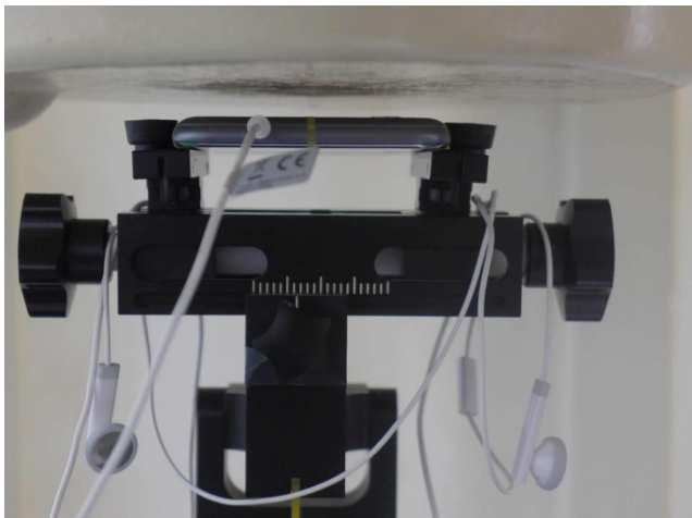
Back with Headset, Test Separation 1 cm
