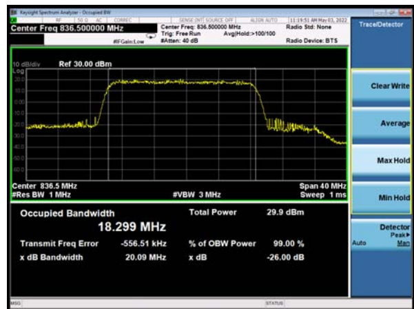
DC_66A-n5A 64QAM 20MHz CH-High
