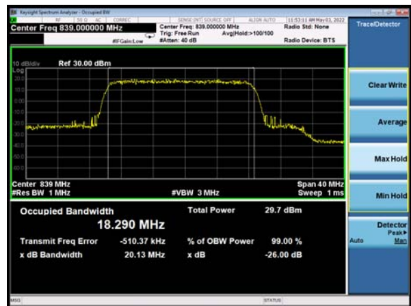
DC_66A-n5A 64QAM 20MHz CH-High
