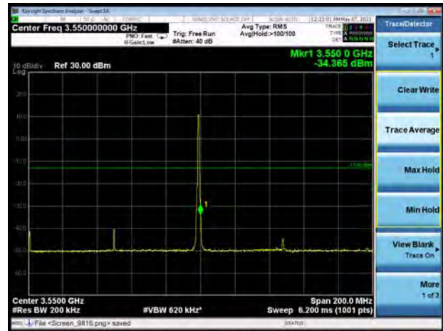
NR n77 subset 1 64QAM 100MHz CH-High 100%RB
