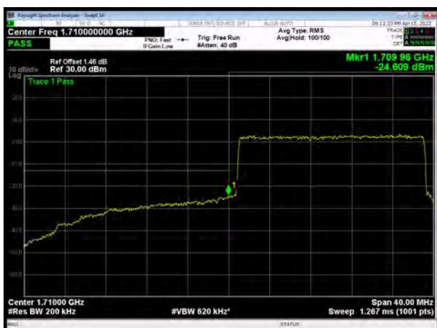
LTE Band 66 64QAM 20MHz CH-Low, 100%RB
