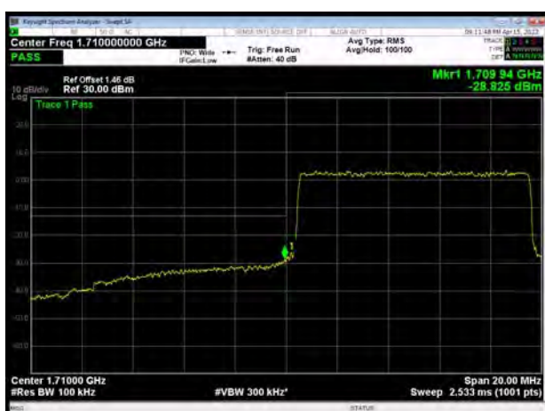
LTE Band 66 64QAM 15MHz CH-Low, 1 RB
