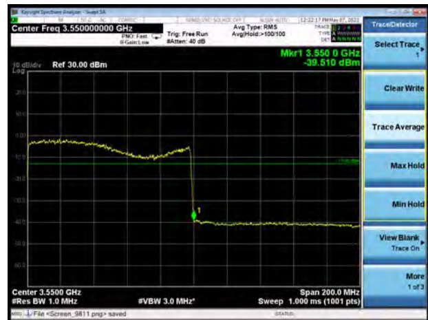
NR n77 subset 1 256QAM 100MHz CH-High 1RB
