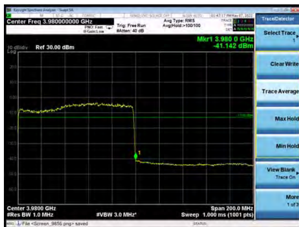
NR n77 subset 2 256QAM 100MHz CH-High 1RB
