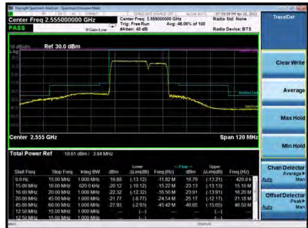
CA_7C 16QAM 20MHz+10MHz CH- High, RB 1
