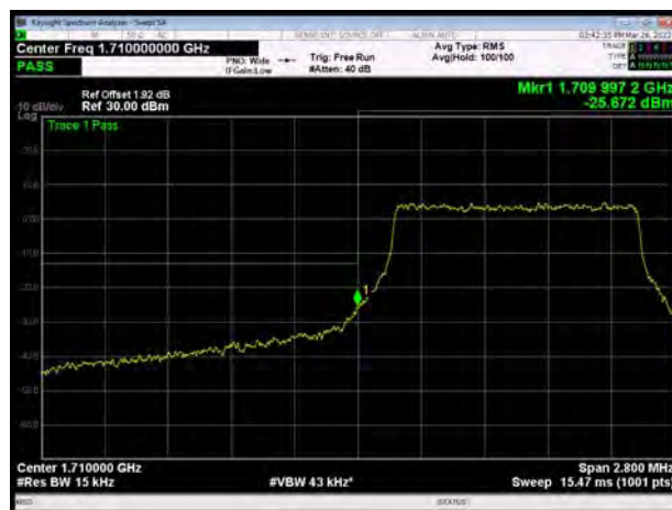
LTE Band 66 16QAM 3MHz CH-Low, 1 RB
