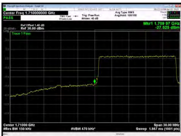
LTE Band 66 64QAM 20MHz CH-Low, 1 RB
