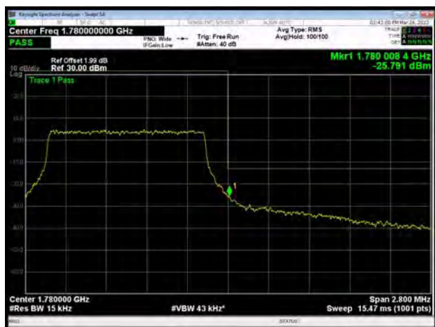
LTE Band 66 16QAM 3MHz CH-High, 1 RB
