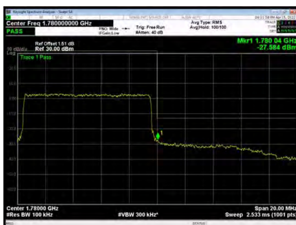
LTE Band 66 64QAM 15MHz CH-High, 1 RB
