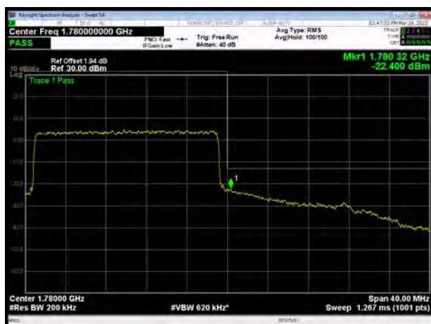
LTE Band 66 QPSK 20MHz CH-High, 100%RB
