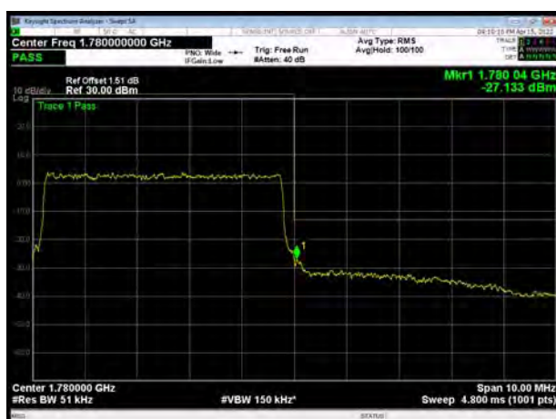
LTE Band 66 64QAM 5MHz CH-High, 100%RB
