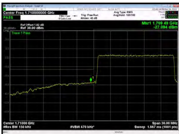
LTE Band 66 16QAM 20MHz CH-Low, 1 RB
