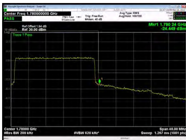
LTE Band 66 16QAM 20MHz CH-High, 100%RB
