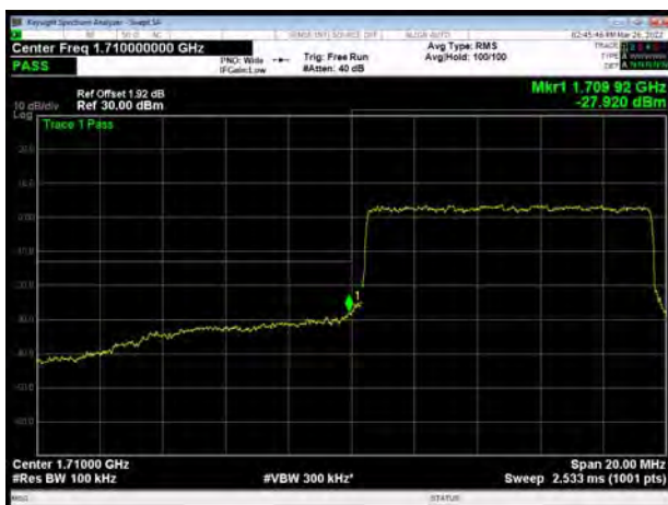
LTE Band 66 16QAM 15MHz CH-Low, 1 RB
