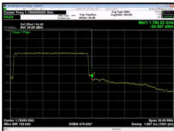
LTE Band 66 QPSK 20MHz CH-High, 1 RB
