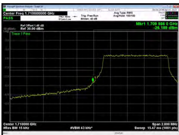
LTE Band 66 64QAM 3MHz CH-Low, 1 RB
