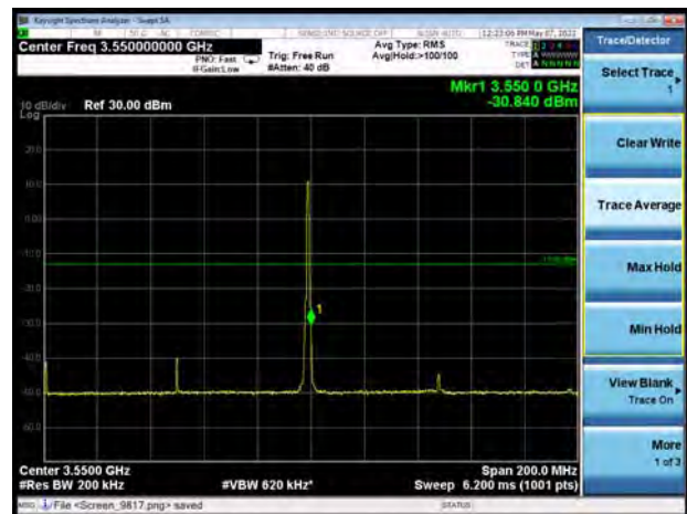
NR n77 subset 1 256QAM 100MHz CH-High 1RB
