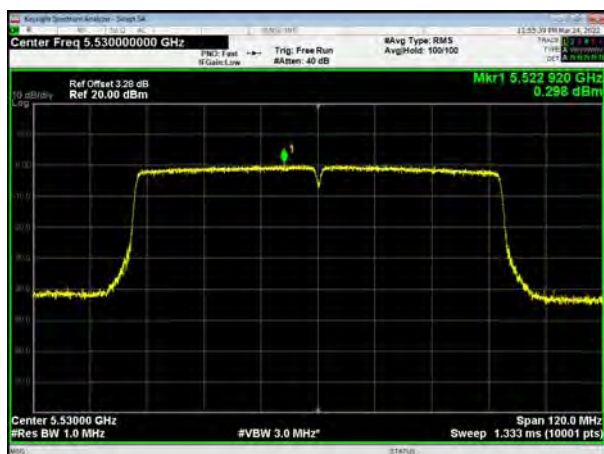
U-NII-2C, 802.11ac VHT80, Channel No.: 138
