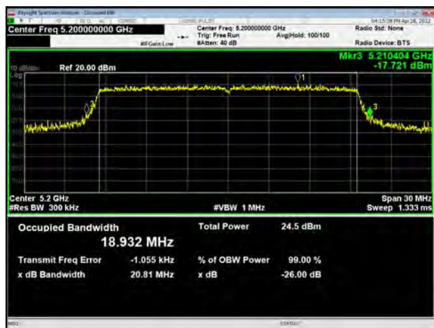
U-NII-1, 802.11ax HE20 Carrier frequency (MHz): 5200
