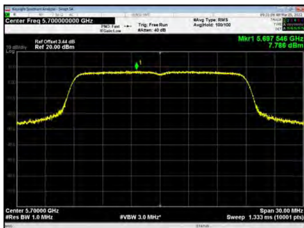
U-NII-2C, 802.11ac VHT20, Channel No.: 140
