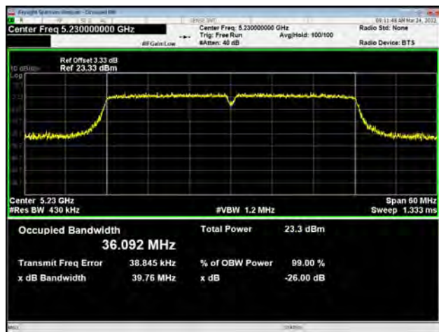
U-NII-1, 802.11ax HE20 Carrier frequency (MHz): 5180
