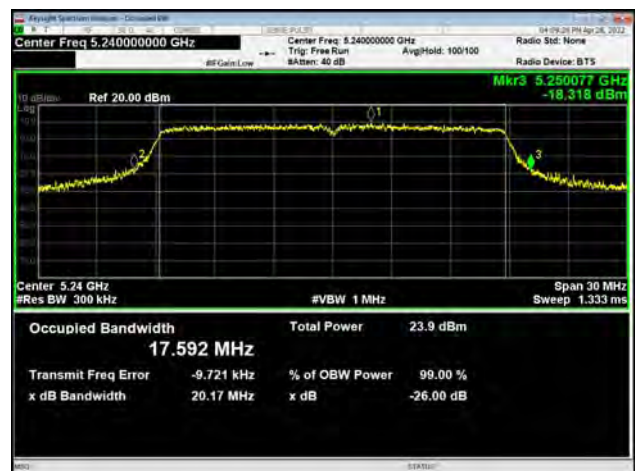
U-NII-1, 802.11n HT20 Carrier frequency (MHz): 5240
