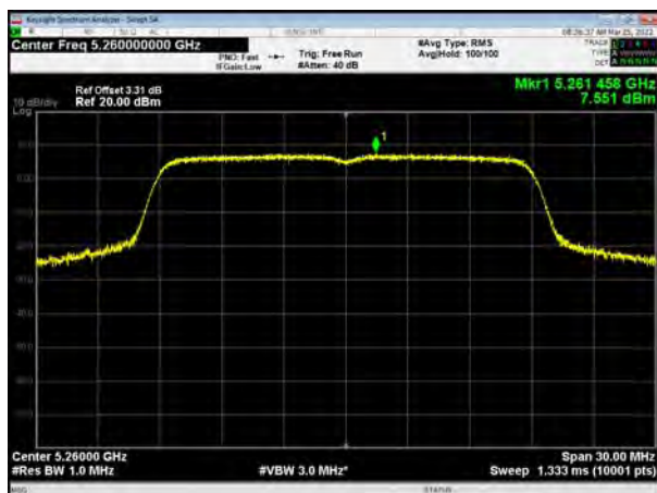
U-NII-2A, 802.11ac VHT20, Channel No.: 60
