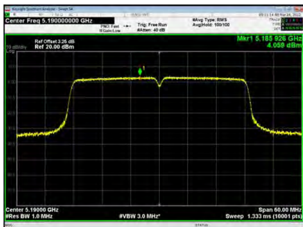
U-NII-1, 802.11ac VHT40, Channel No.: 38
