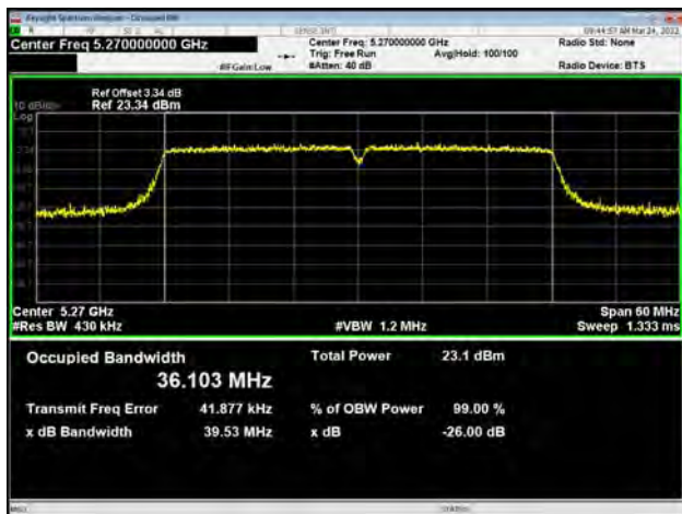
U-NII-2A, 802.11n HT40 Carrier frequency (MHz): 5310
