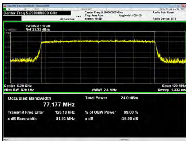
U-NII-2C, 802.11n HT20 Carrier frequency (MHz): 5500
