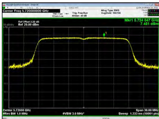
U-NII-2C, 802.11ac VHT80, Channel No.: 106
