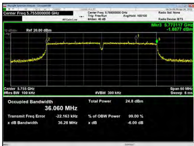
U-NII-3, 802.11n HT40 Carrier frequency (MHz): 5795
