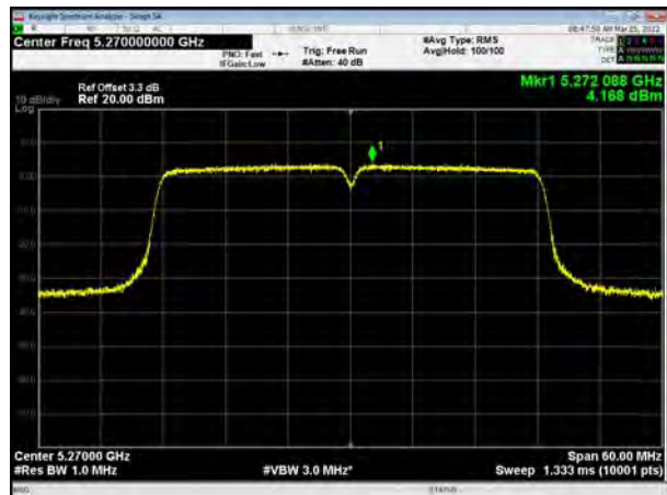
U-NII-2A, 802.11ac VHT40, Channel No.: 62
