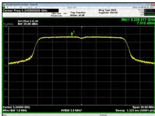
U-NII-1, 802.11ac VHT20, Channel No.: 48
