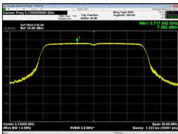
U-NII-2C, 802.11ac VHT80, Channel No.: 106
