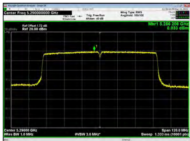
U-NII-2A, 802.11ac VHT80, Channel No.: 58
