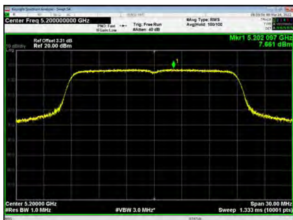
U-NII-1, 802.11ac VHT20, Channel No.: 48
