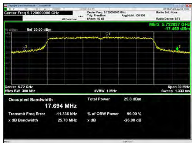
U-NII-2C, 802.11n HT20 Carrier frequency (MHz): 5720
