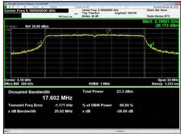
U-NII-1, 802.11n HT20 Carrier frequency (MHz): 5200
