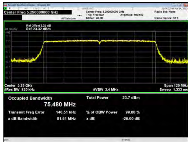
U-NII-2A, 802.11ax HE40 Carrier frequency (MHz): 5270
