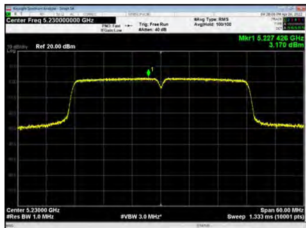
U-NII-1, 802.11ac VHT80, Channel No.: 42
