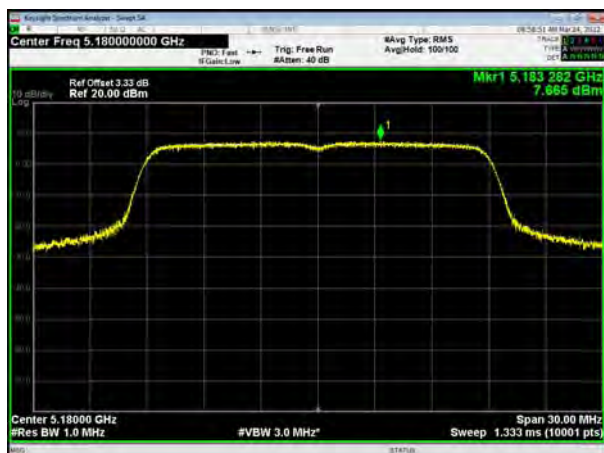
U-NII-1, 802.11ac VHT20, Channel No.: 40
