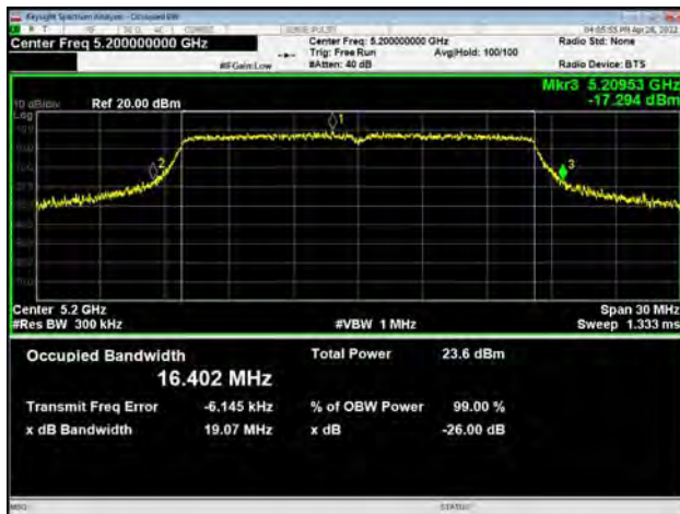
U-NII-1, 802.11a Carrier frequency (MHz): 5240
