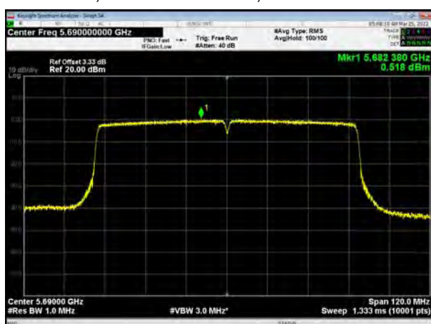
U-NII-2C, 802.11ac VHT80, Channel No.: 138
