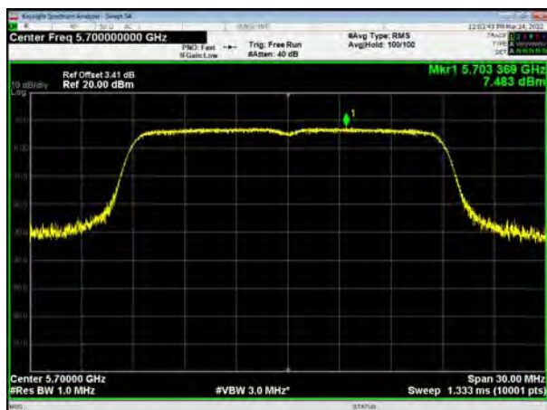
U-NII-2C, 802.11ac VHT20, Channel No.: 140
