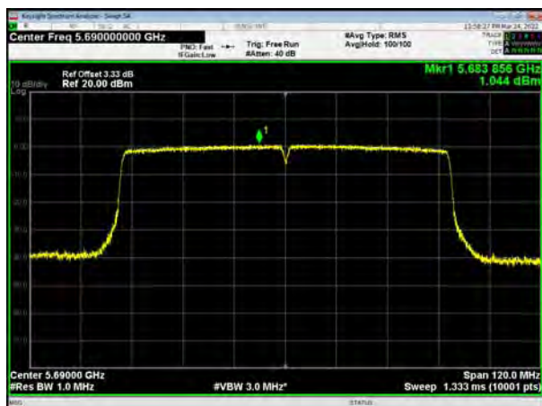
U-NII-2C, 802.11ac VHT80, Channel No.: 138
