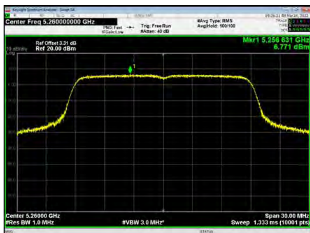
U-NII-2A, 802.11ac VHT20, Channel No.: 60
