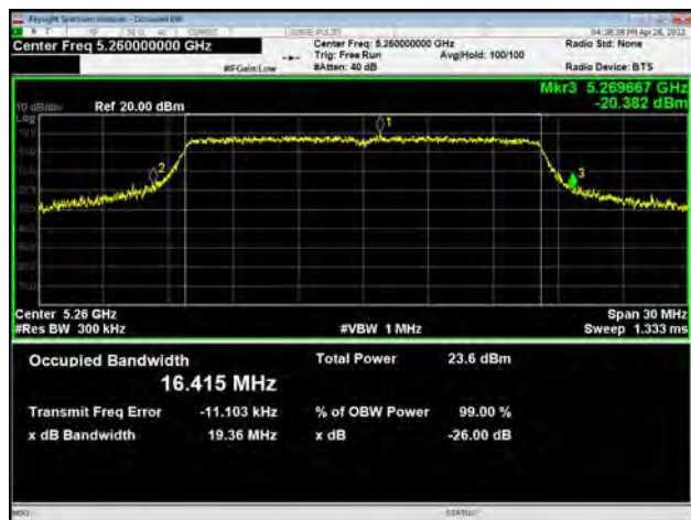
U-NII-2A, 802.11a Carrier frequency (MHz): 5300
