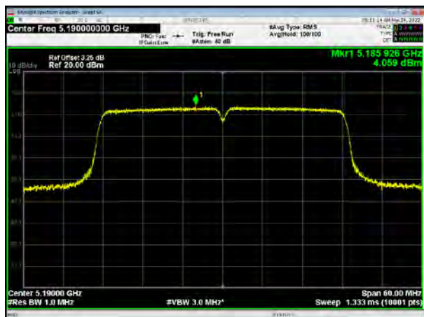
U-NII-1, 802.11ac VHT40, Channel No.: 38
