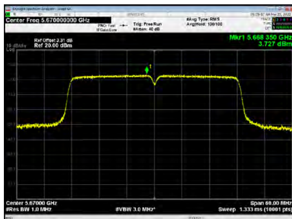
U-NII-2C, 802.11ac VHT40, Channel No.: 142
