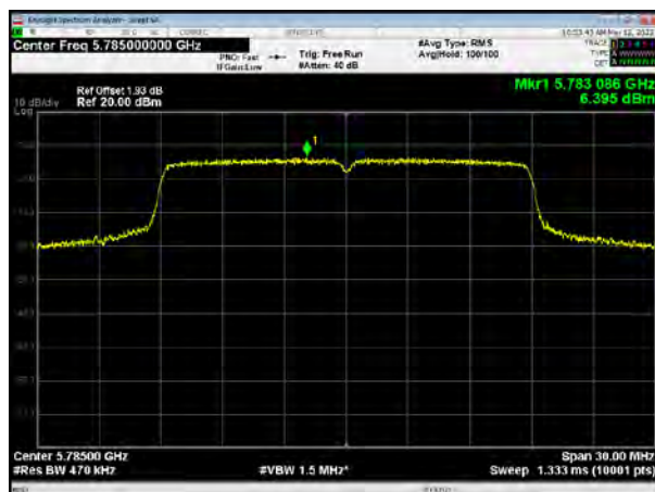
U-NII-3, 802.11ac VHT20, Channel No.: 165
