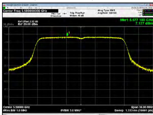
U-NII-2C, 802.11ac VHT20, Channel No.: 140
