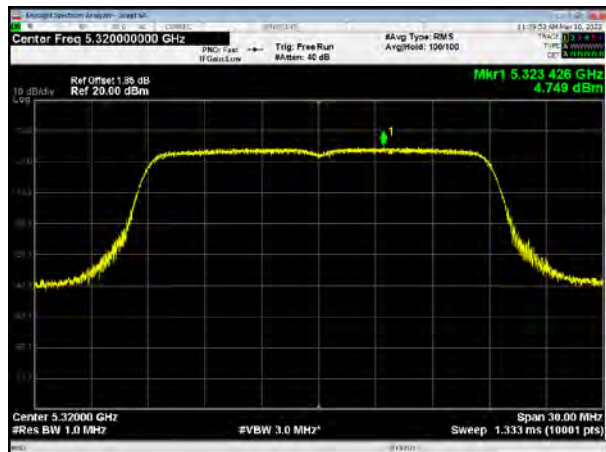
U-NII-2A, 802.11ac VHT80, Channel No.: 58
