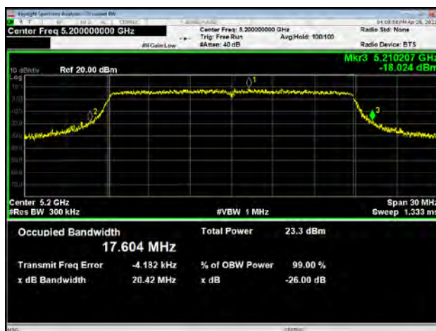
U-NII-1, 802.11n HT20 Carrier frequency (MHz): 5240
