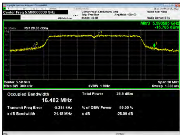
U-NII-2C, 802.11a Carrier frequency (MHz):5700
