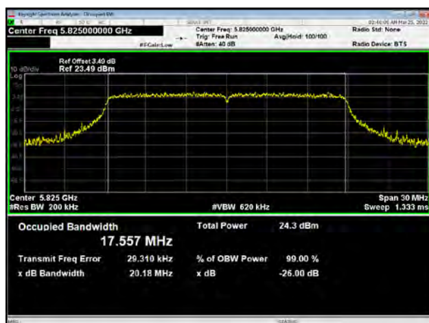
U-NII-3, 802.11n HT20 Carrier frequency (MHz): 5825
