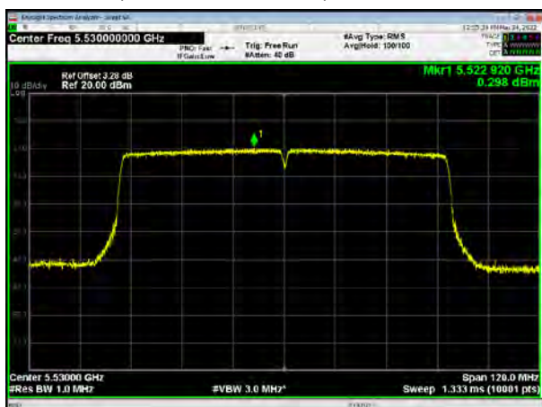
U-NII-2C, 802.11ac VHT80, Channel No.: 138
