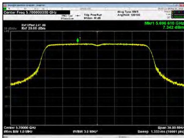
U-NII-2C, 802.11ac VHT20, Channel No.: 140
