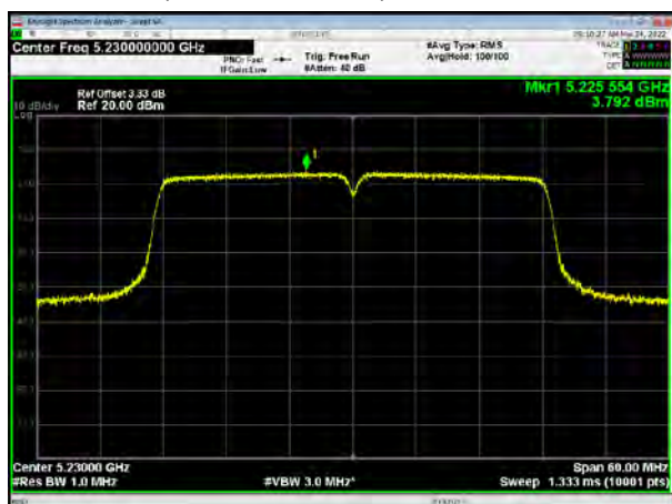
U-NII-1, 802.11ac VHT40, Channel No.: 38
