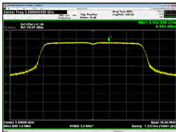
U-NII-2C, 802.11ac VHT20, Channel No.: 116
