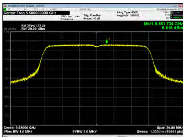
U-NII-2C, 802.11ac VHT20, Channel No.: 140
