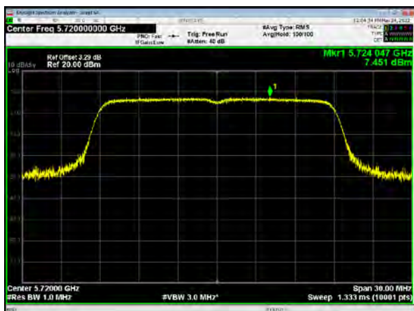
U-NII-2C, 802.11ac VHT80, Channel No.: 106
