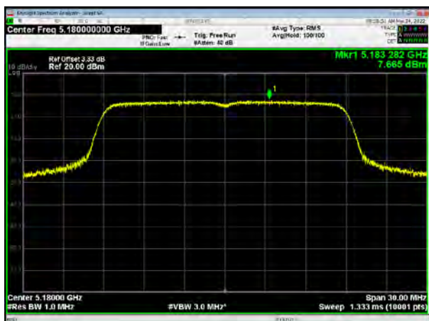
U-NII-1, 802.11ac VHT20, Channel No.: 40
