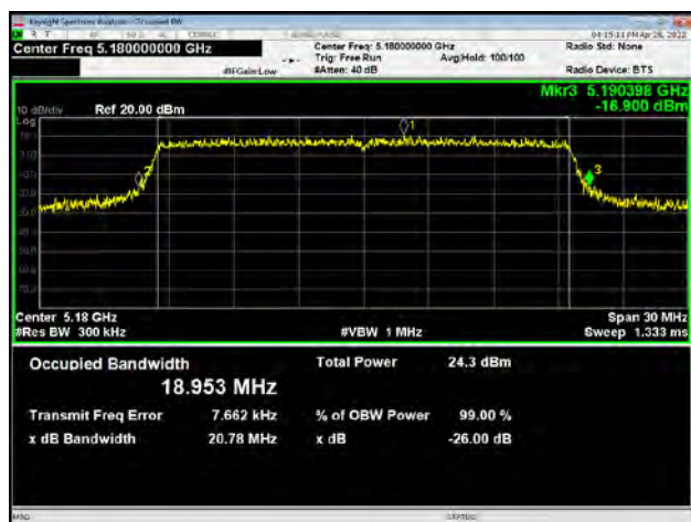
U-NII-1, 802.11ax HE20 Carrier frequency (MHz): 5200
