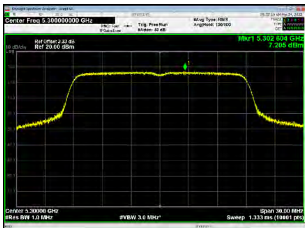
U-NII-2A, 802.11ac VHT20, Channel No.: 60
