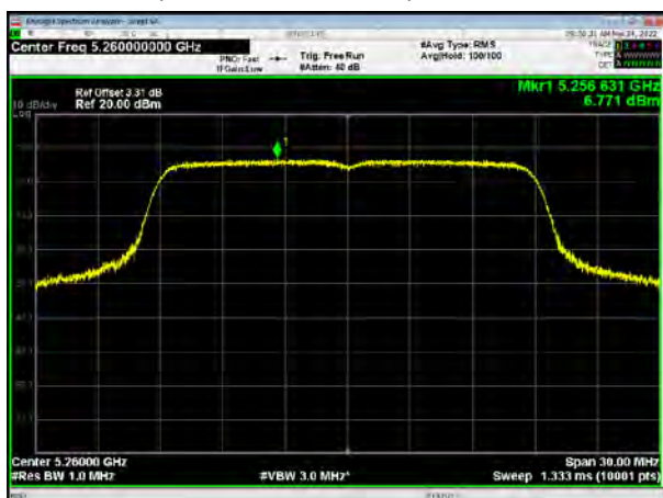
U-NII-2A, 802.11ac VHT20, Channel No.: 60
