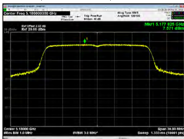
U-NII-1, 802.11ac VHT20, Channel No.: 40
