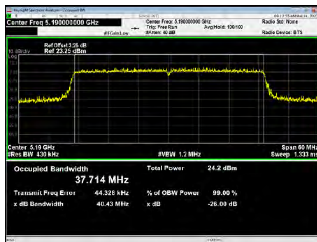
U-NII-1, 802.11ax HE40 Carrier frequency (MHz): 5230
