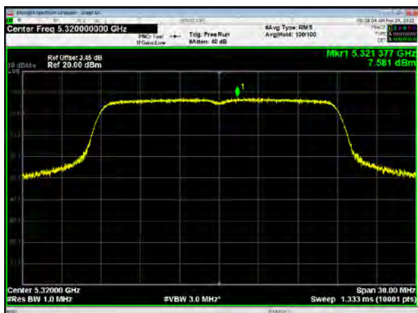
U-NII-2A, 802.11ac VHT80, Channel No.: 58
