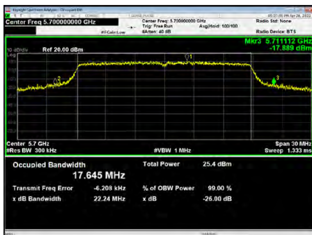
U-NII-2C, 802.11n HT20 Carrier frequency (MHz):5720
