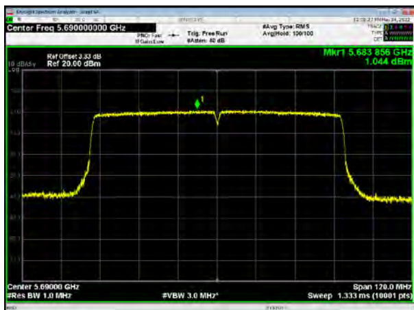
U-NII-2C, 802.11ac VHT80, Channel No.: 138
