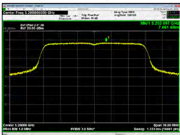
U-NII-1, 802.11ac VHT20, Channel No.: 48
