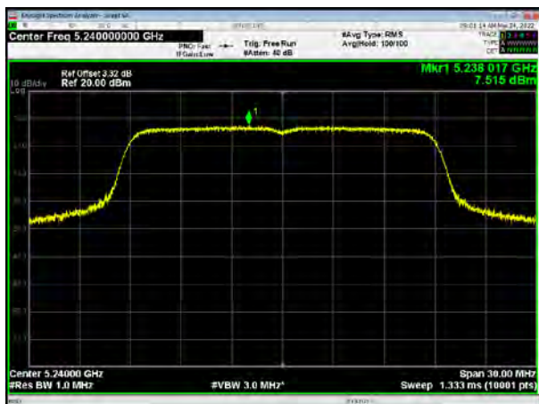
U-NII-1, 802.11ac VHT20, Channel No.: 48
