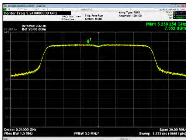
U-NII-1, 802.11ac VHT20, Channel No.: 48
