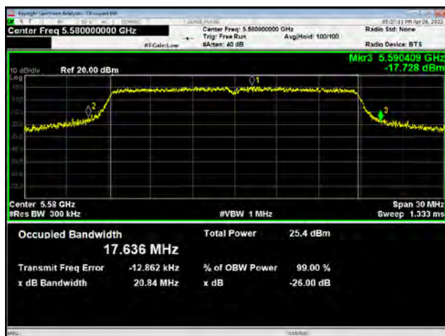
U-NII-2C, 802.11n HT20 Carrier frequency (MHz):5700
