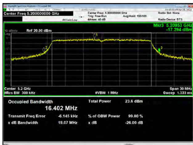
U-NII-1, 802.11a Carrier frequency (MHz): 5240
