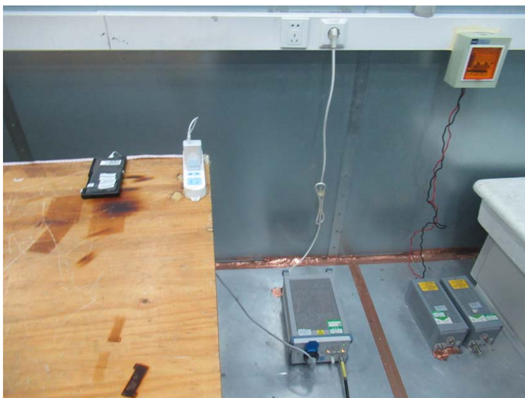
Picture 2 Conducted Emission Test Setup
