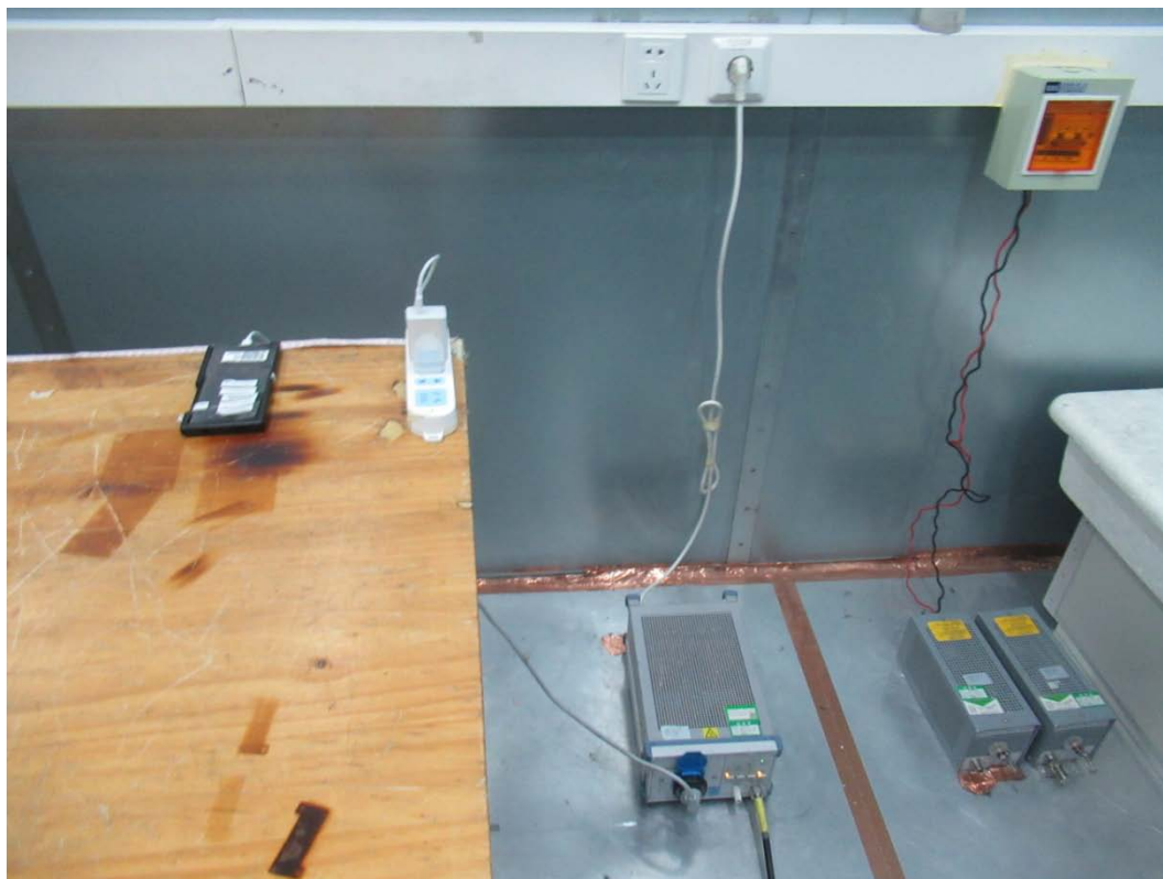
Picture 2 Conducted Emission Test Setup
