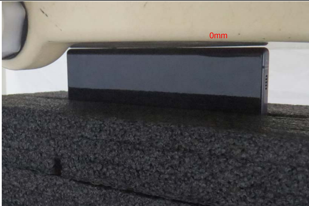
Picture 15: Left Edge, the distance from handset to the bottom of the Phantom is 0mm
