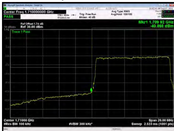
LTE Band 4 16QAM 15MHz CH-Low, 1 RB
