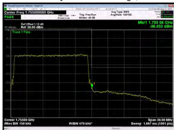
LTE Band 4 64QAM 20MHz CH-High, 1 RB
