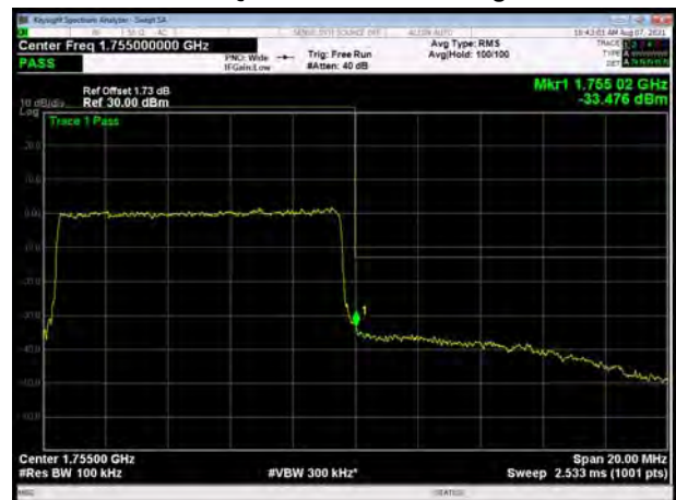
LTE Band 4 16QAM 15MHz CH-High, 1 RB
